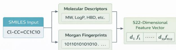
Figure 2. Feature engineering pipeline illustrating the transformation of SMILES representations into a unified 522-dimensional molecular feature vector through the combination of physicochemical descriptors and Morgan fingerprint features.
