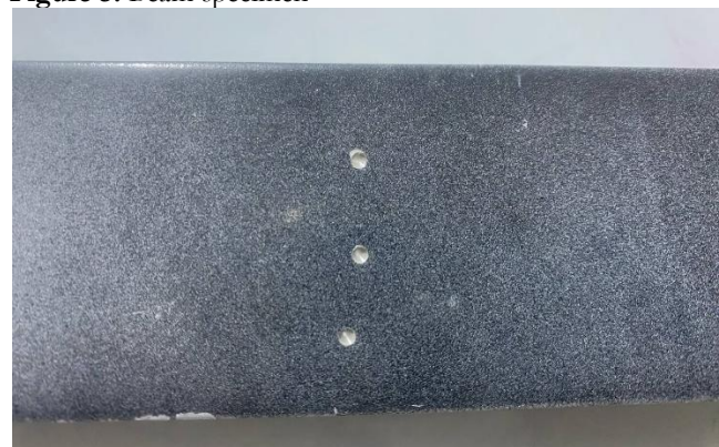
Figure 6. Holes drilled on the top surface
