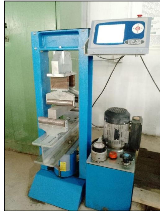
Figure 3. Experimental setup for the four-point bending test
