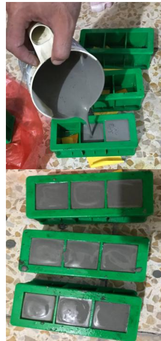
Figure 4. Preparation of 50 mm grout cubes in molds for compressive strength testing (ASTM C109/C109M).
