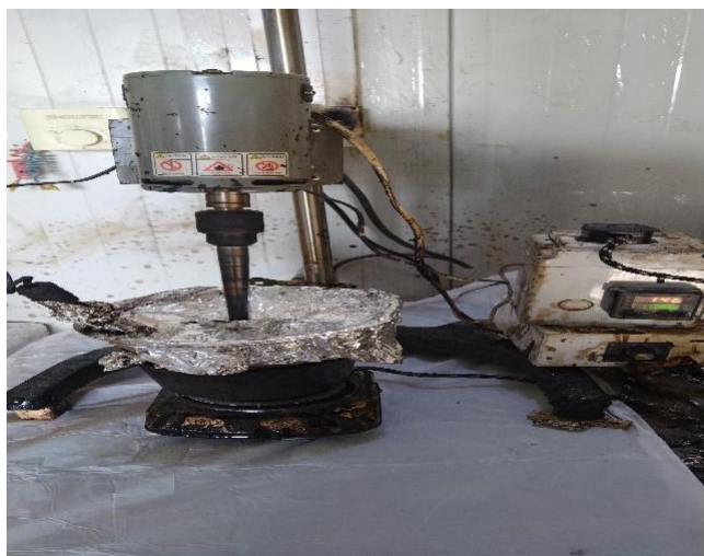
Figure 2. Shear mixer machine used in the preparation of the modified binder.
