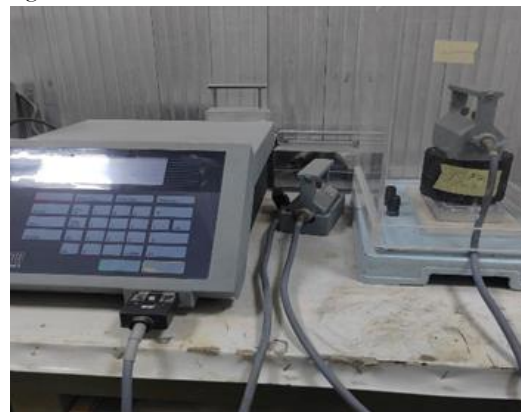
Figure 3. The QTM-500 Quick Thermal Conductivity Meter used for measuring the thermal conductivity of materials.
