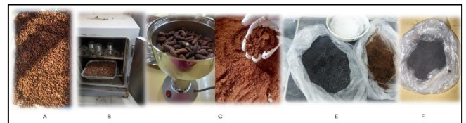
Figure 2. Sequential processing stages for thermally treated date seed powder: (a) washing and air drying, (b) oven drying at 70°C, (c) grinding, and sieving, (d) pyrolysis at 450°C, (e) activation at 650°C.
