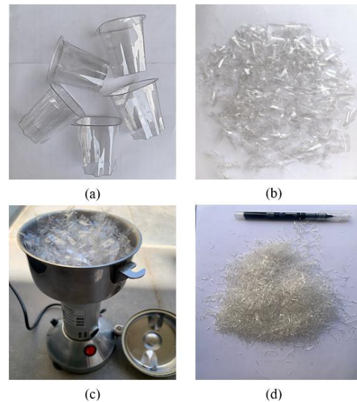
Figure 4. Procedure to prepare crushed PET: (a) Collecting disposable plastic cups; (b) Plastic cups after cutting; (c) Crushing plastic; (d) Crushed plastic
