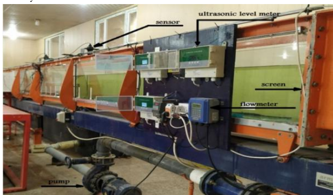
Figure 2. The used flume (Civil Engineering Department, Engineering College, Babylon University)
