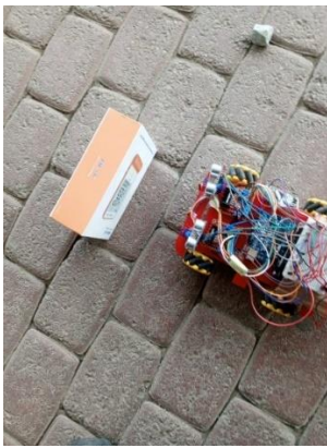
Figure 10c. Testing of the prototype with 1 obstacle placed at the front on a rough surface
