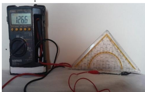
Figure 11. shows how to measure the change in angle with a change in resistance.
