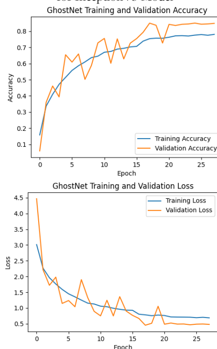
Figure 4. Training And Validation Curves of Accuracy and Loss for GhostNet Model
