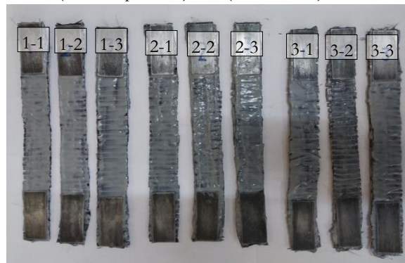
Figure 7. Steel-CFRP strengthening coupons: 1 layer, 2 layers and 3 layers.
