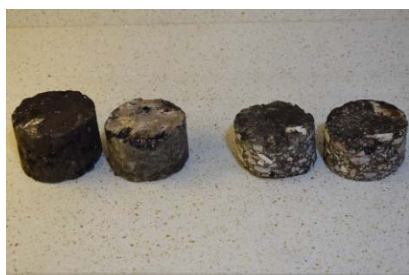
(d) Aged and Unaged Tested Samples Figure 11. The Standard Steps of Marshall Compaction Process
