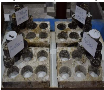
d. Compacted Slabs after Coring
