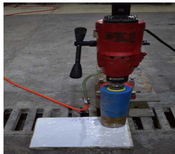
a. Preparing Slabs for Coring
