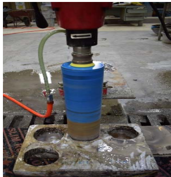
b. Cored Samples Per Slab
