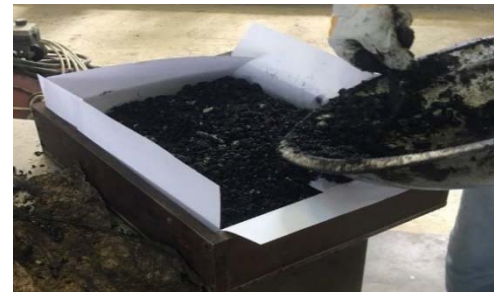
(c) Mould Greasing and Mix Pouring
