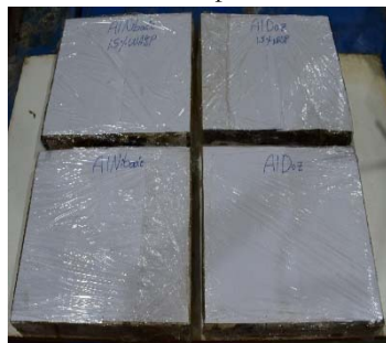
c. Prepared Slabs by Roller Compaction
