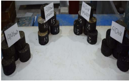
Figure 8. The Prepared Reference and Modified Samples of the Marshall Method
