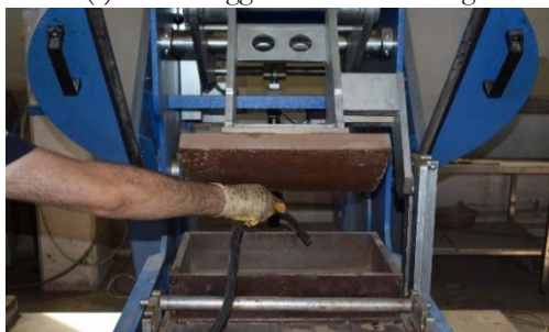
(b) Mould Cleaning by air pressure
