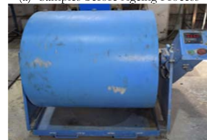
(b) Abrasion Assessment in Los Angeles Device
