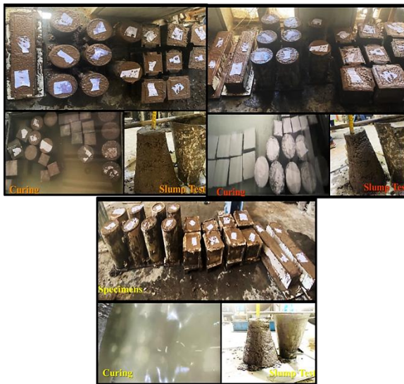
Figure 5. Zeolite blended cement specimens design.
