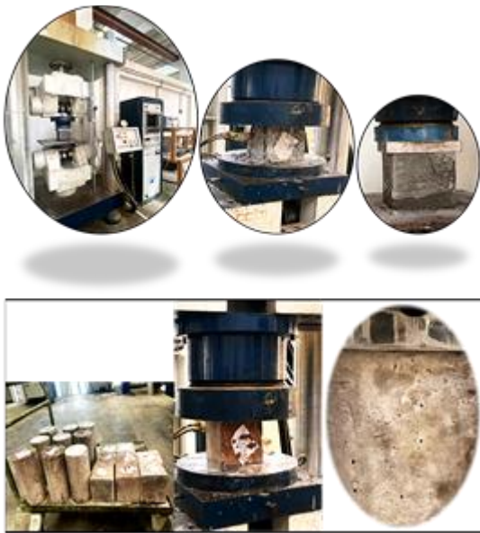
Figure 8. Compression strength of normal and zeo-concrete test.
