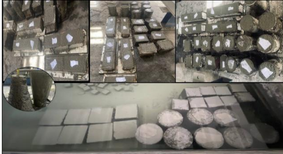
Figure 4. Plain concrete mix production and sample preparation.
