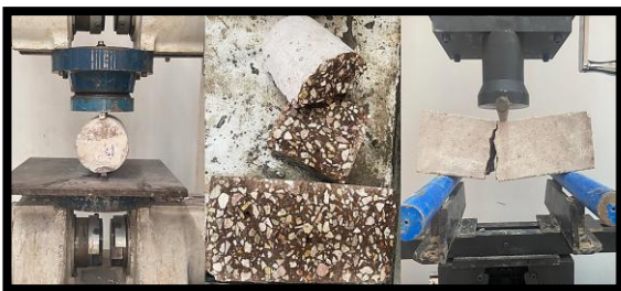
Figure 9. Tensile and flexural strength of zeo-concrete tests.
