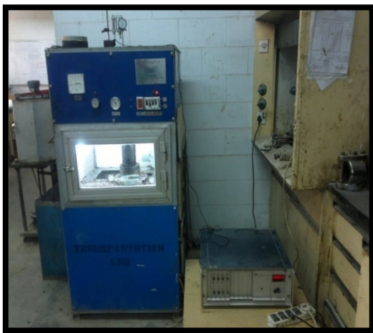
Figure 3 Permanent Deformation Specimens during the Test (Highway Material lab, University of Baghdad)
