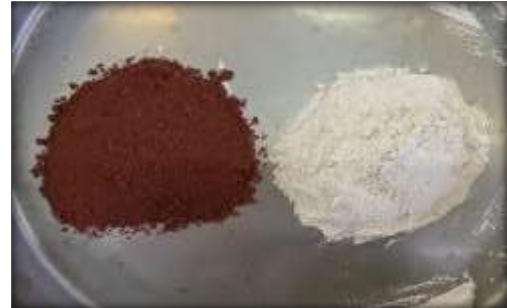
Figure (2): filler type used in this search left: Iron oxide III, right: limestone.
