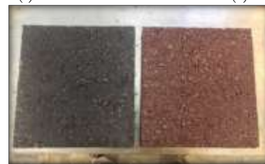
Figure (7): (a) fine mix with 10% Iron oxide III (b) coarse mix with 6% oxide III (c) fine mix: left with 6% limestone Right: with 6% Iron oxide III
