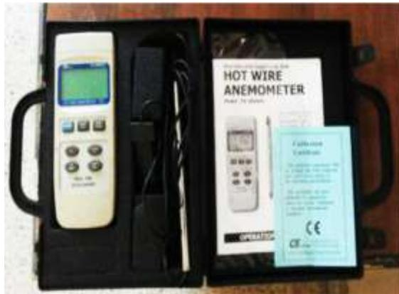
Figure (5): Air velocity hot wire Anemometer (model yk-2005AH).
