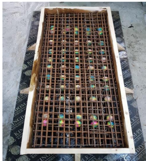
Plate 3 Bubble Slab with Shear Reinforcement (multi-leg)
