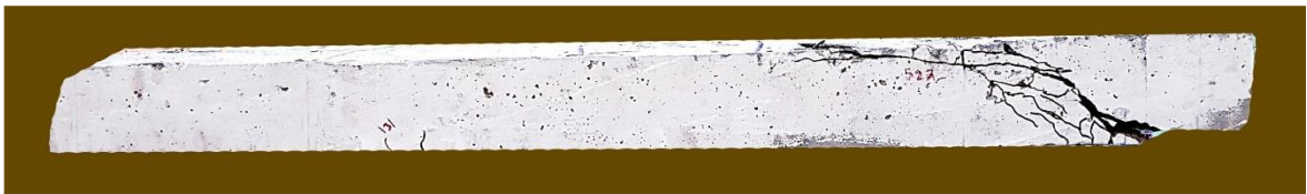
Plate 12 Crack pattern and mode of failure of bubbled slab (G4-S3)
