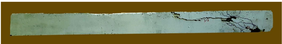
Plate 16 Crack pattern and mode of failure of bubbled slab (G5-S3)
