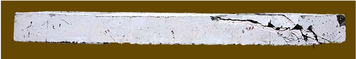
Plate 11 Crack pattern and mode of failure of bubbled slab (G4-S2)
