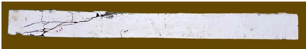
Plate 6 Crack pattern and mode of failure of bubbled slab (G2-S1)
