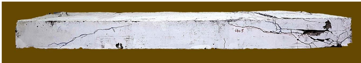
Plate 7 Crack pattern and mode of failure of bubbled slab (G2-S2)
