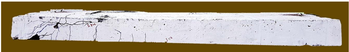
Plate 13 Crack pattern and mode of failure of bubbled slab (G4-S4)
