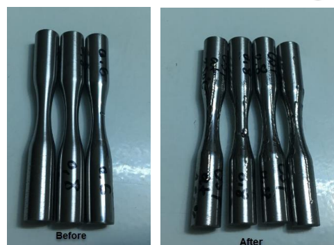
Figure (9): the fatigue specimens before and after ultrasonic peening treatment.
