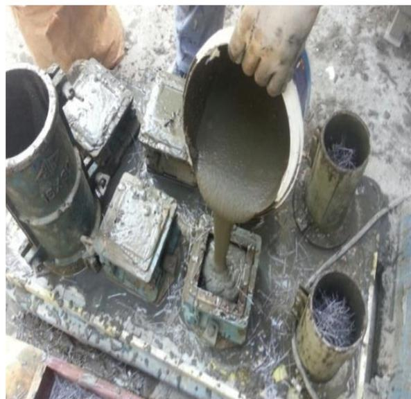
**Figure (2):** Slurry infiltration through steel-fiber by using external vibration [4].
