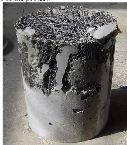
**Figure (3):** Failed in preparation due to loss of the fluidity of slurry [4].
