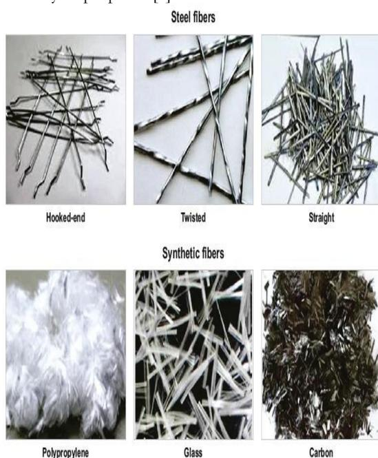
**Figure (1):** type of discrete fiber [3].
