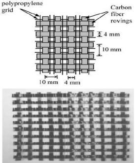
Figure (4): textile carbon fiber [8].
