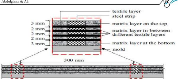
Figure (8): Cross section of four-layer BTRC plates during fabrication [7].
