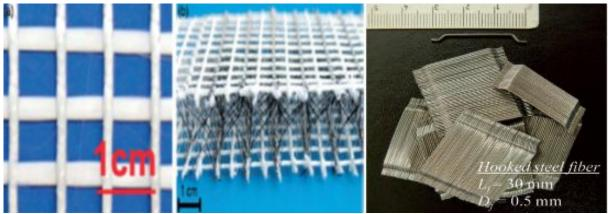
Figure (9): the shape and geometry of (2D, 3D) textile AR glass fiber, and hooks end steel [13].
