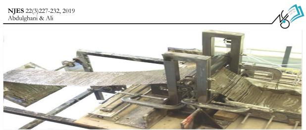
Figure (6): the fabrics dragged out through the cement bath [10].
