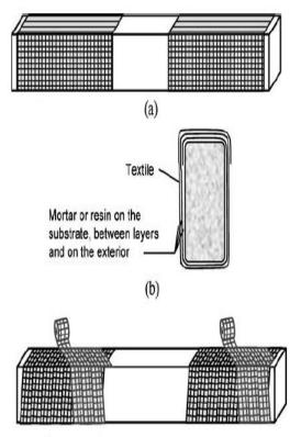
Figure (5): Applying textile-reinforced-mortar in the shear spans: (a) normal cover, (b) more layers of textile with mortar [8].
