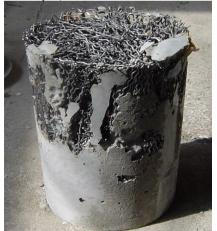
Figure (3): Failed in preparation due to loss of the fluidity of slurry [4].
