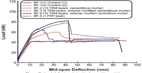
Figure (7): Load-deflection relationship for tested beams [11].
