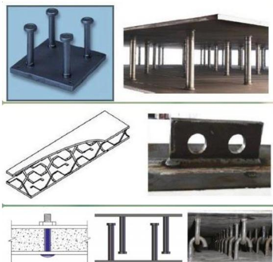
Figure (1): Divers types of mechanical shear connectors.
