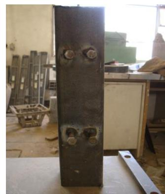
a) Steel section with shear connectors
