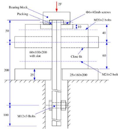
a) Test arrangement for bars in pure shear
