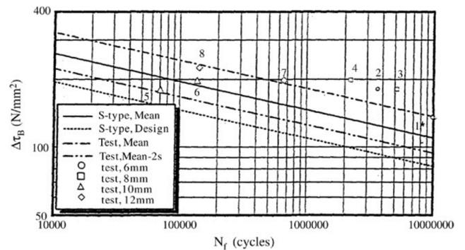
c) Diagrammatic S versus N relation for bars subjected to pure shear.
