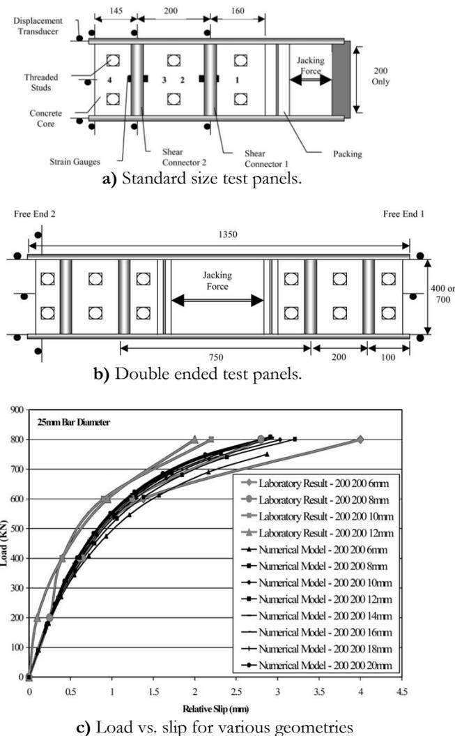
Figure (7): Push-out tests used by [Clublely et al., 1999].
