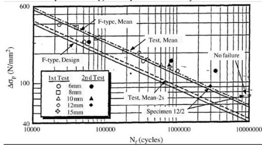
b) Diagrammatic S versus N relation for free plate-bars system.
