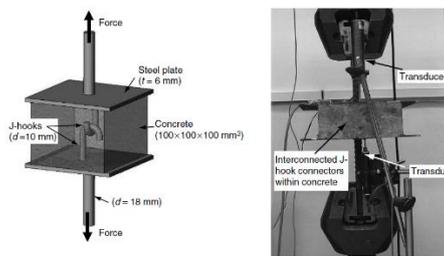
a) Tensile test arrangement
