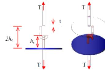
b) Tensile tests on J-hook connector
