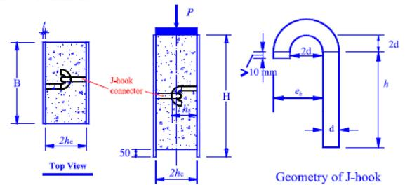
a) Push-out test setup and specimen geometry.
