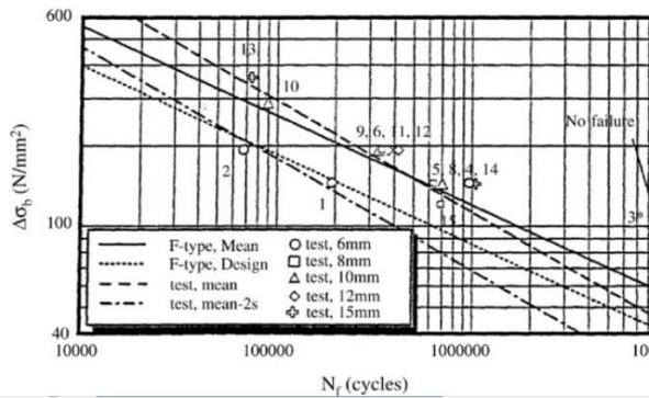
b) S-N lines for bars in bending.
