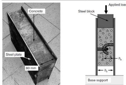
b) Push-out shear test arrangement
