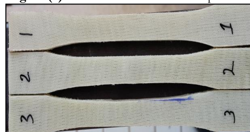
Figure (9): The three samples of lamination for tensile test
