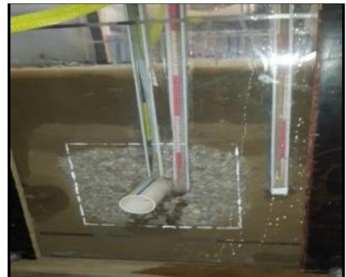
**Figure (2):** The location of piezometer to measure entrance resistance.
