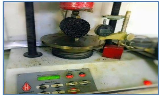
Plate (6): Details of indirect tensile test and sample tested
