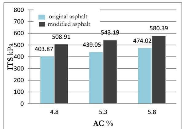
Figure (4): Effect of modified asphalt binder content on its 25°C.
