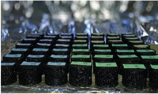
Plate (5): Specimens for permeability test
