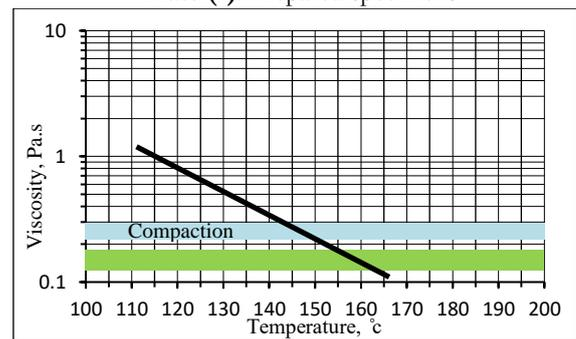
Figure (2): Viscosity-temperature chart for asphalt 40/50
