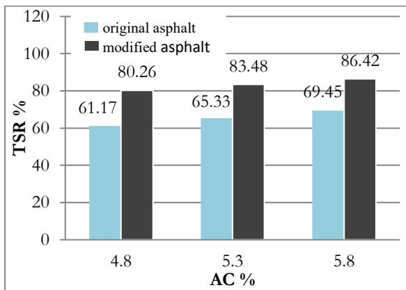
Figure (6): Effect of modified asphalt binder content on TSR%
