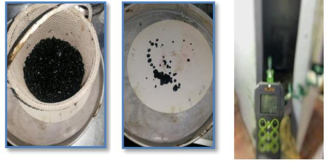
Plate (3): Asphalt draindown test
