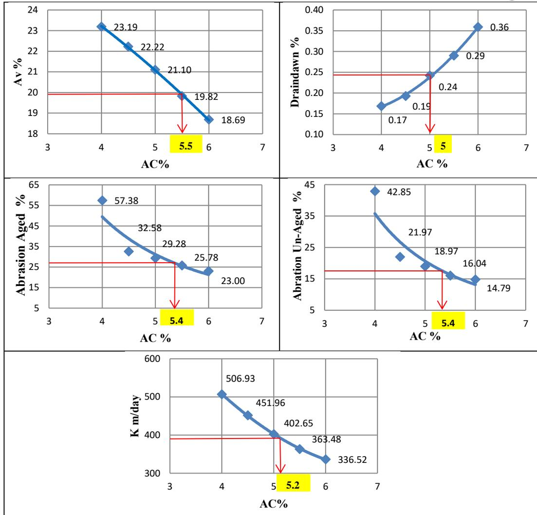
Figure (3): Asphalt binder ratio with criteria
