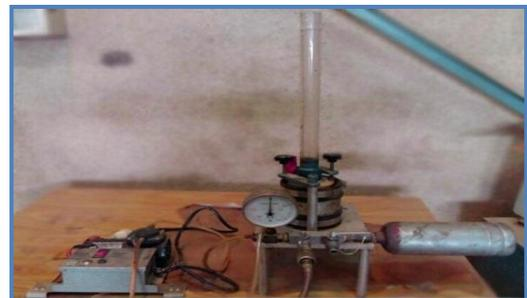
Plate (4): Hydraulic conductivity apparatus
