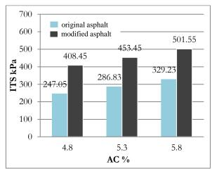
**Figure (5):** Effect of modified asphalt binder content on its 60°C after 24 hr. (frees/thaw)
