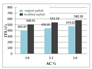
**Figure (4):** Effect of modified asphalt binder content on its 25°C.
