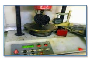
**Plate (6):** Details of indirect tensile test and sample tested
