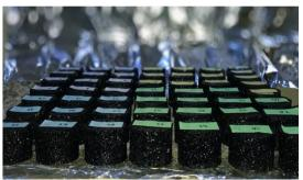
Plate (5): Specimens for permeability test
