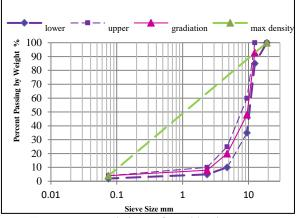
**Figure (1):** Gradations of combined aggregate (NMAS 12.5 mm) used in this work
