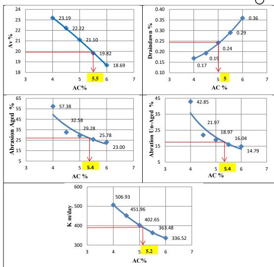
Figure (3): Asphalt binder ratio with criteria
