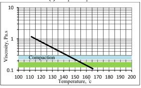
**Figure (2):** Viscosity-temperature chart for asphalt 40/50
