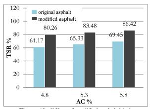
**Figure (6):** Effect of modified asphalt binder content on TSR%
