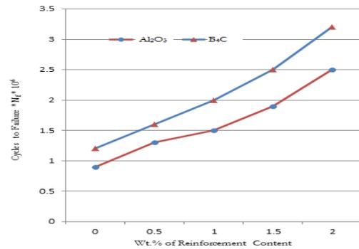
**Fig. (8):** Cycles to failure versus ceramic particles weight fraction wt% under 50 MPa
