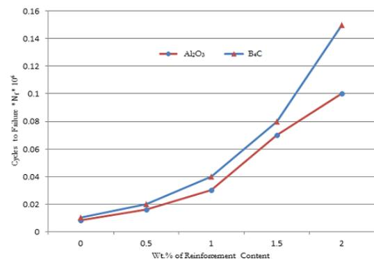
**Fig. (10):** Cycles to failure versus Ceramic particles weight fraction wt% under 400 MPa
