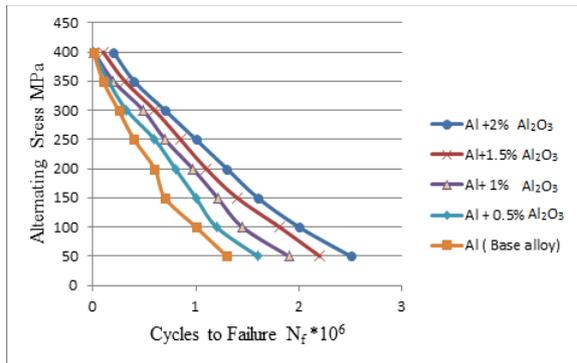
**Fig (12):** Alternating stress versus cycles to failure for AMCs strengthened with Al<sub>2</sub>O<sub>3</sub> particles
