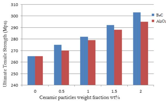
**Fig. (6):** Shows ultimate tensile strength versus ceramic particles weight fraction
