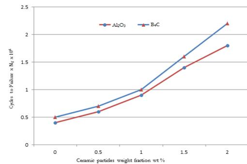
**Fig. (9):** Cycles to failure versus ceramic particles weight fraction wt% under 250
