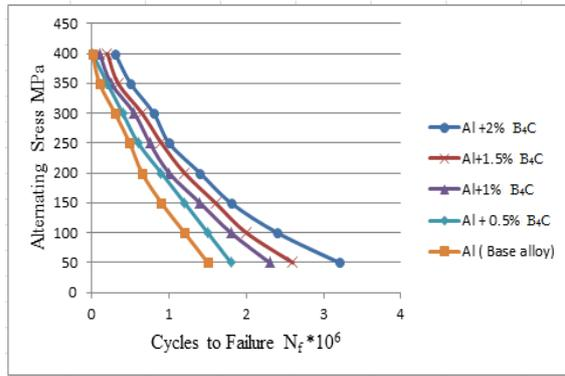
**Fig (11):** Alternating stress versus cycles to failure for AMCs strengthened with B<sub>4</sub>C particles
