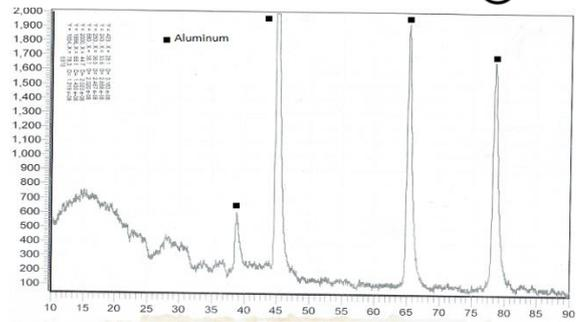
Fig. (3): Explains X-ray diffraction pattern for nano Al<sub>2</sub>O<sub>3</sub> reinforced AMCs
