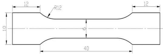
Fig. (1): shows tensile sample
