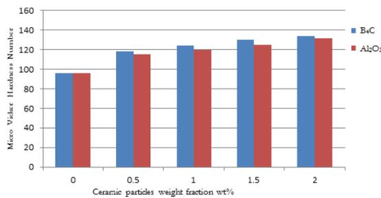
**Fig. (7):** Shows micro-Vickers number versus ceramic particles weight fraction
