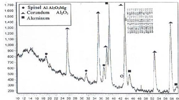
Fig. (5): Shows X-ray diffraction pattern for nanoparticles Al<sub>2</sub>O<sub>3</sub> reinforced AMCs.
