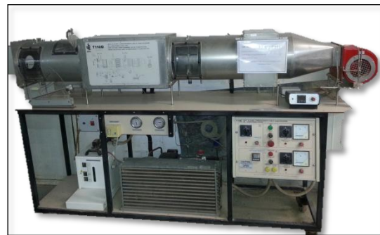
Figure 2: Air duct used in the experimental work
