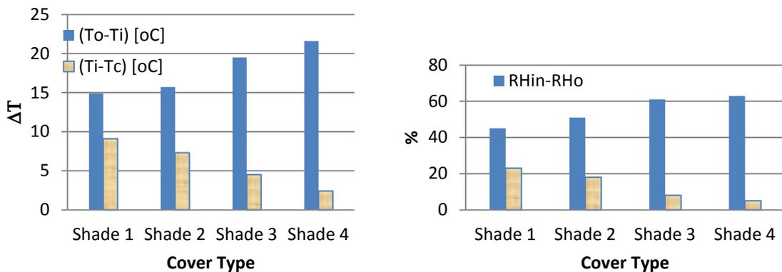
Figure (11) Comparison of temperature and relative humidity differences between greenhouse and outdoor for different covers
