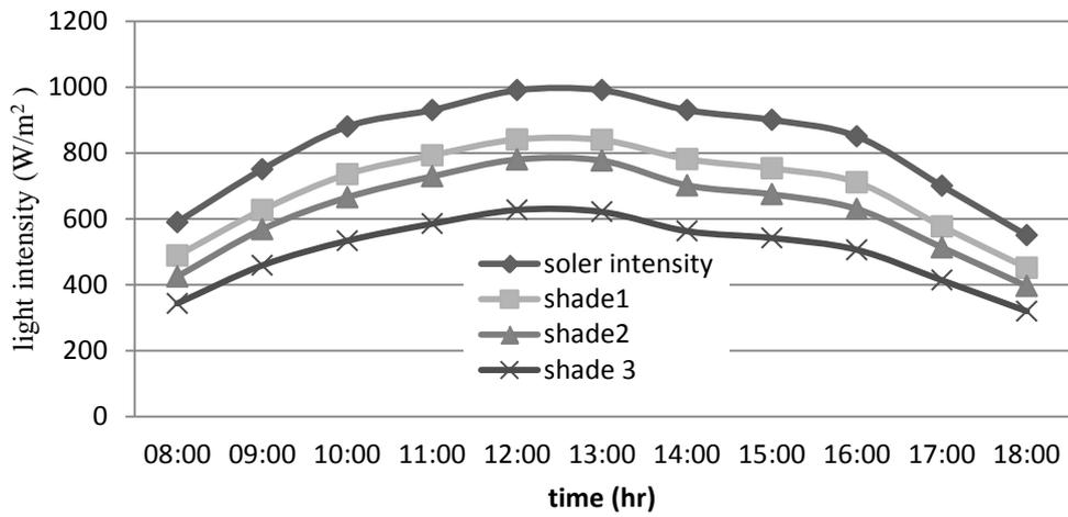
Figure 6: Measuring solar Intensity for differnet greenhouse cover
