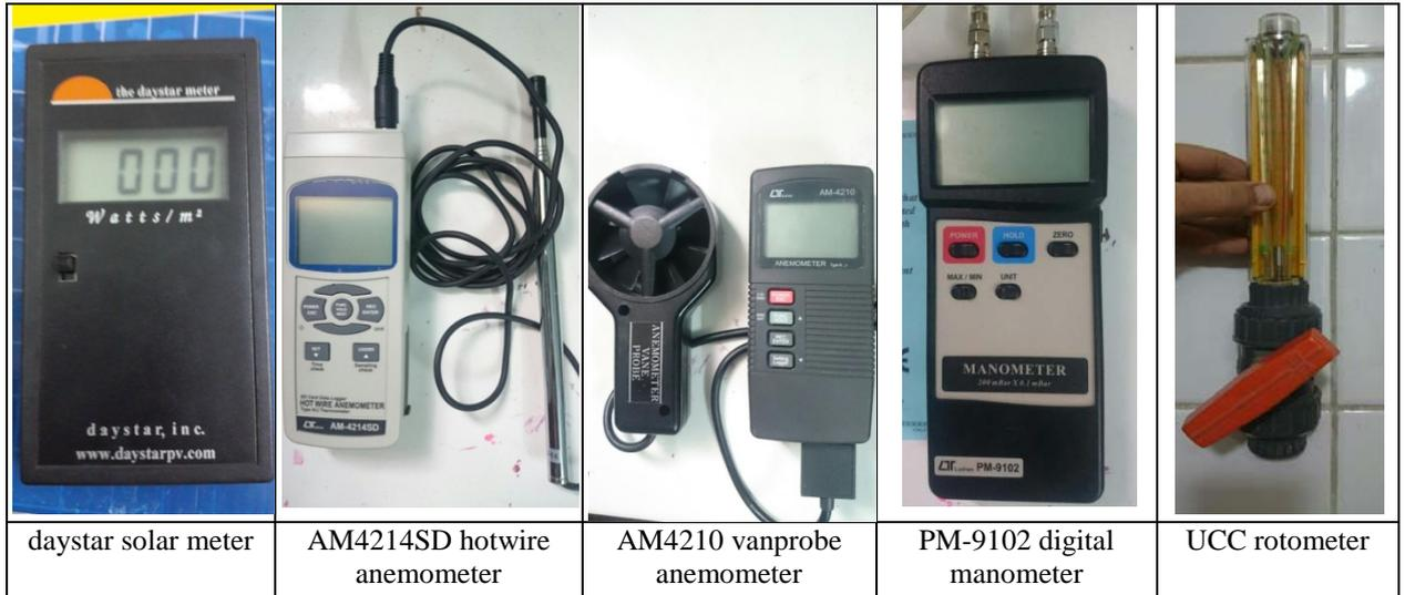
Figure 5: the Instruments used in the work
