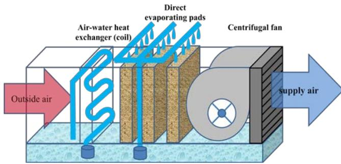
Figure 2: shows the schematic diagram of cooler
