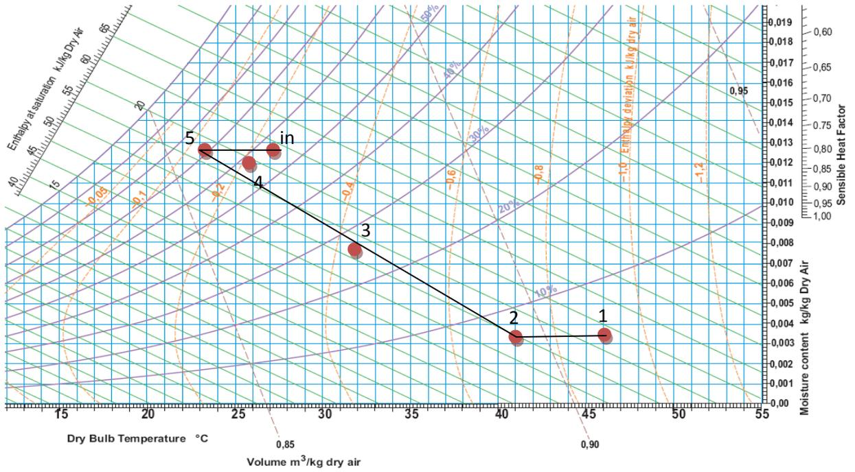
Figure 9: Psychrometric representation of indirect direct evaporative cooling of greenhouse with shade 3.
