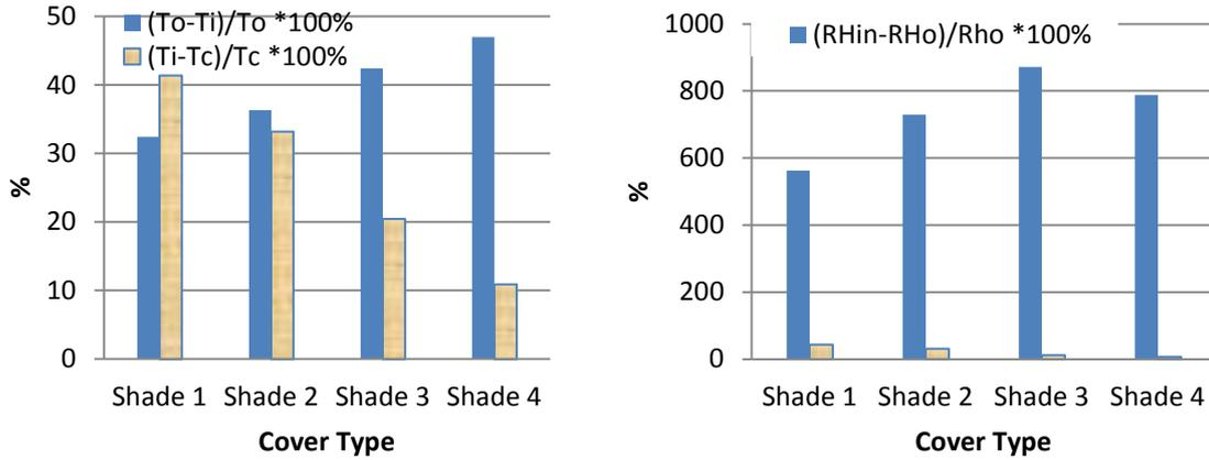
**Figure 12:** Comparison of percentage differences of temperature and relative humidity greenhouse with outdoor and outlet of the cooler for different covers
