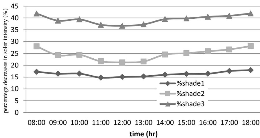
Figure 7: Percentege reduction of solar Intensity for differnet greenhouse cover
