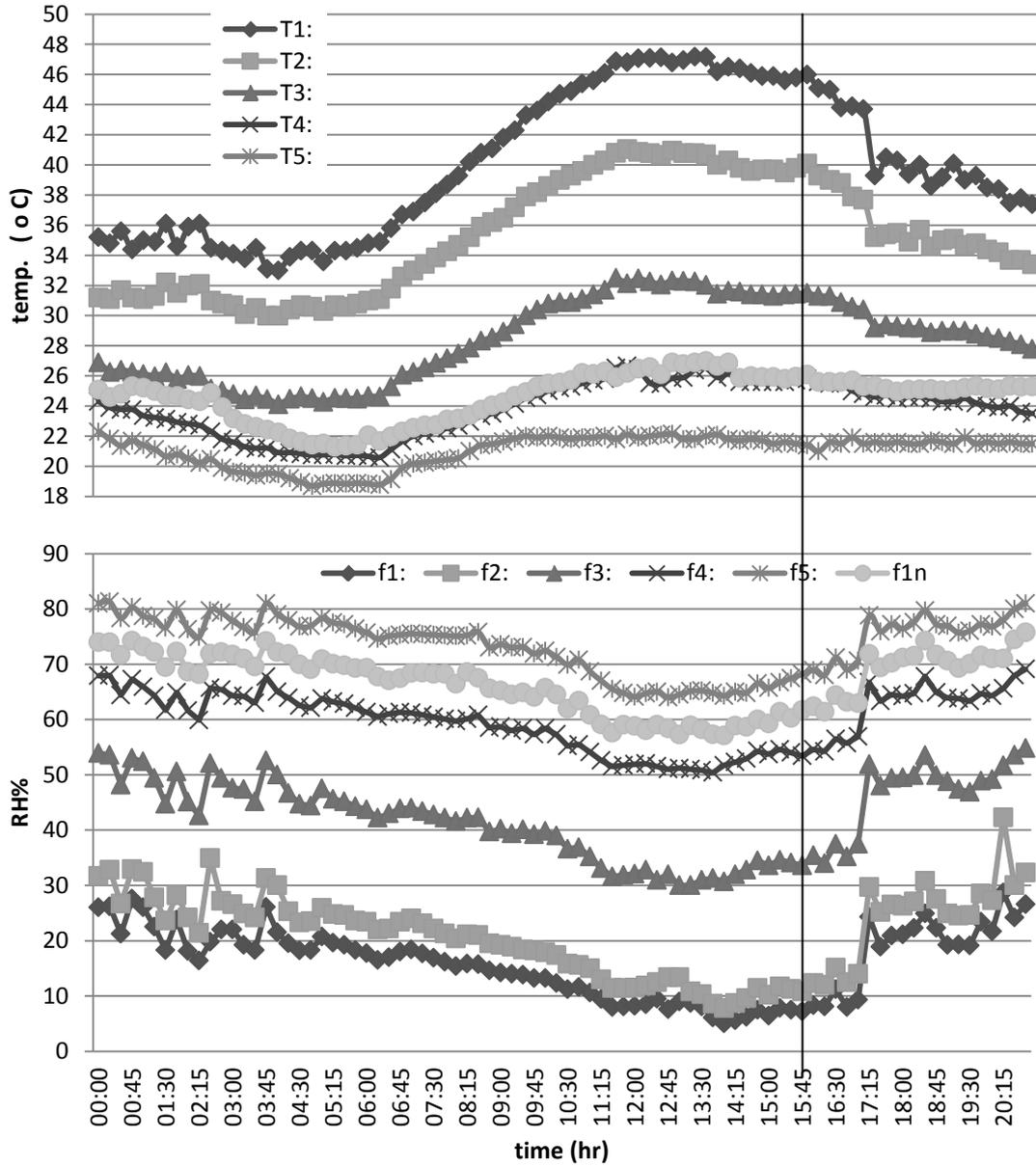
**Figure 8:** The temperatures and values of percentage relative humidity plotted versus time for different stages of indirect-direct evaporative cooling and inside greenhouse.
