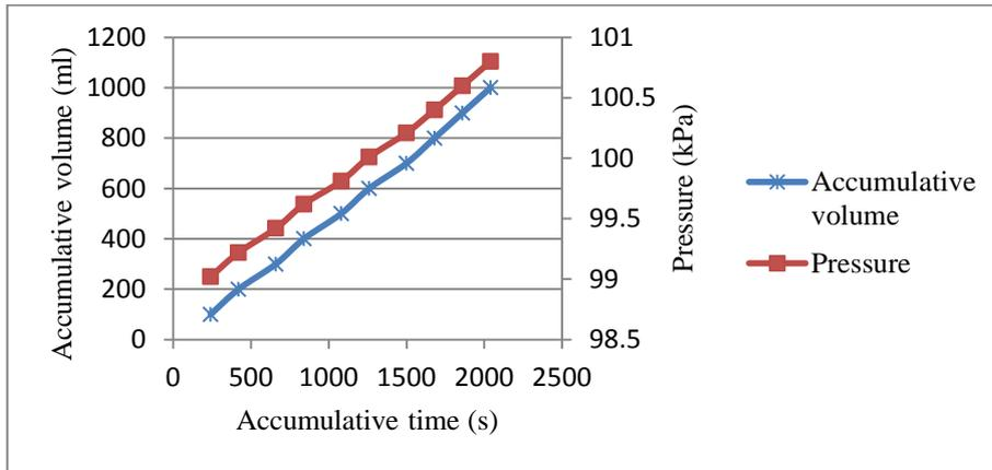
Figure 8: Accumulative volume and pressure with accumulative time for 50 gram NaOH concentration,  $45^\circ\text{C}$  inlet water temperature and  $42^\circ\text{C}$  ambient temperature.
