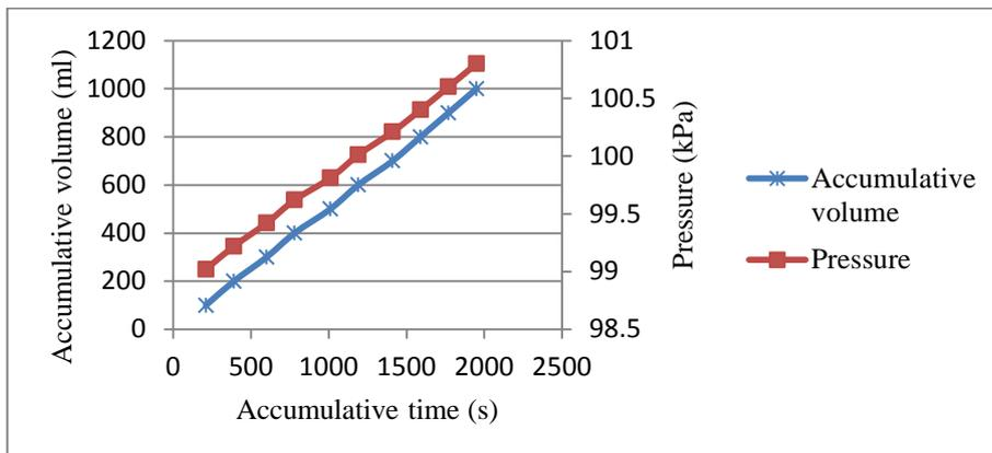
Figure 9: Accumulative volume and pressure with accumulative time for 50 gram NaOH concentration,  $50^\circ\text{C}$  inlet water temperature and  $43^\circ\text{C}$  ambient temperature.
