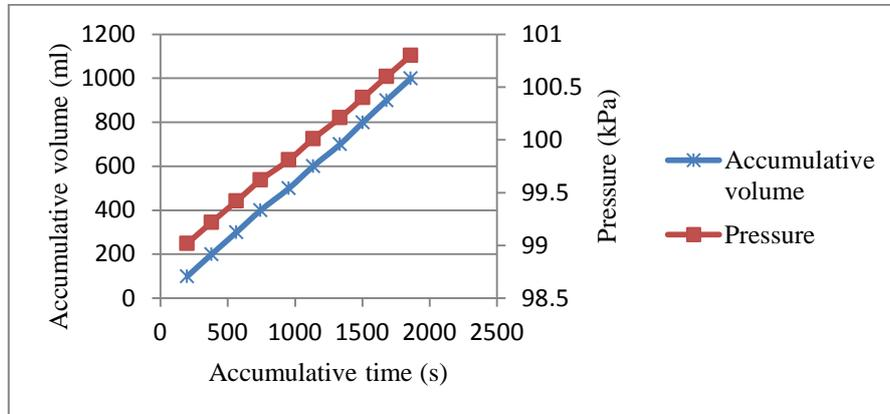
Figure 11: Accumulative volume and pressure with accumulative time for 50 gram NaOH concentration, 60 ° C inlet water temperature and 45°C ambient temperature.
