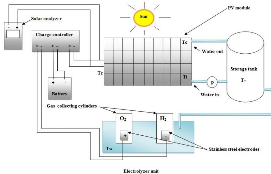
**Figure 1:** Schematic diagram of the experimental set-up with thermocouples locations.
