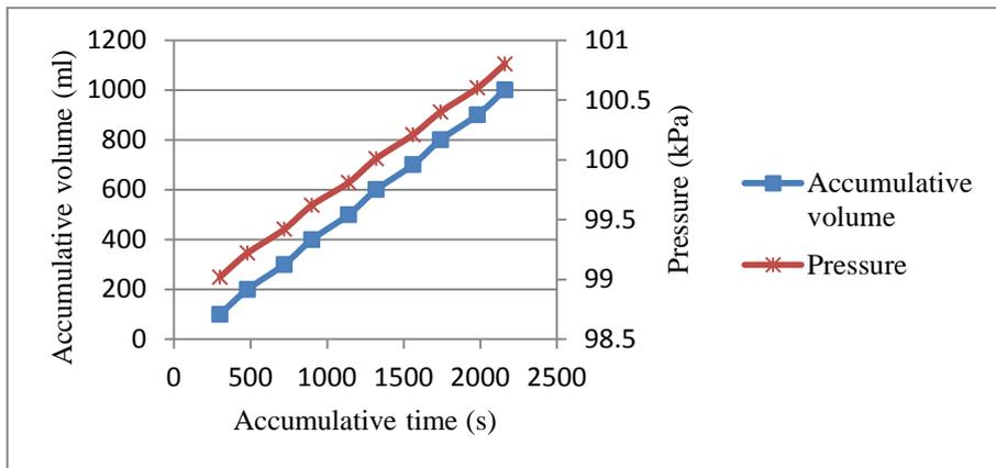
Figure 7: Accumulative volume and pressure with accumulative time for 50 gram NaOH concentration, 40 °C inlet water temperature and 38°C ambient temperature.
