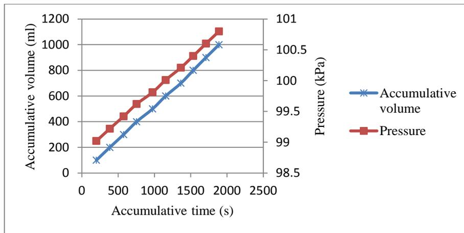
**Figure 10:** Accumulative volume and pressure with accumulative time for 50 gram NaOH concentration,  $55^\circ\text{C}$  inlet water temperature and  $45^\circ\text{C}$  ambient temperature.
