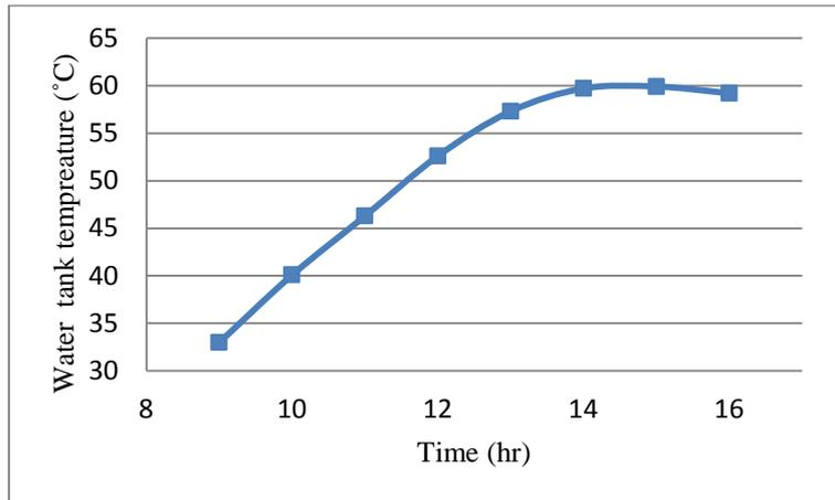
Figure 3: Temperature of the storage tank with time on 10<sup>th</sup> of October 2015.
