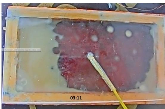
**Figure 24 :** Photographic Observation Showing Propagation of Melting of Wax without Metal Foam
