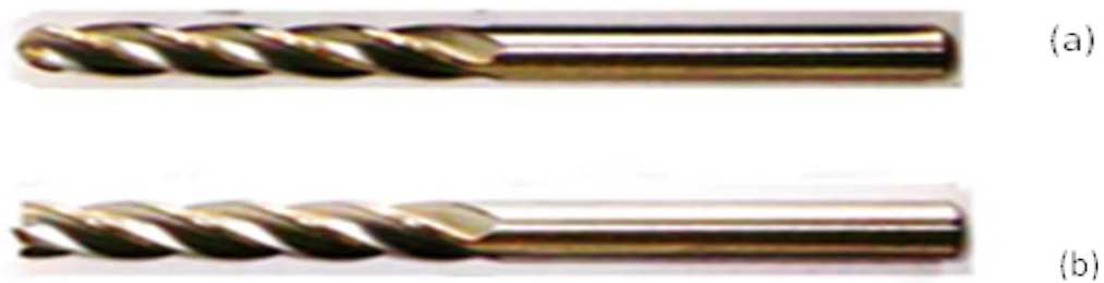
Figure 6: The cutting tools used, (a) ball end cutting tool (b) flat end cutting tool
