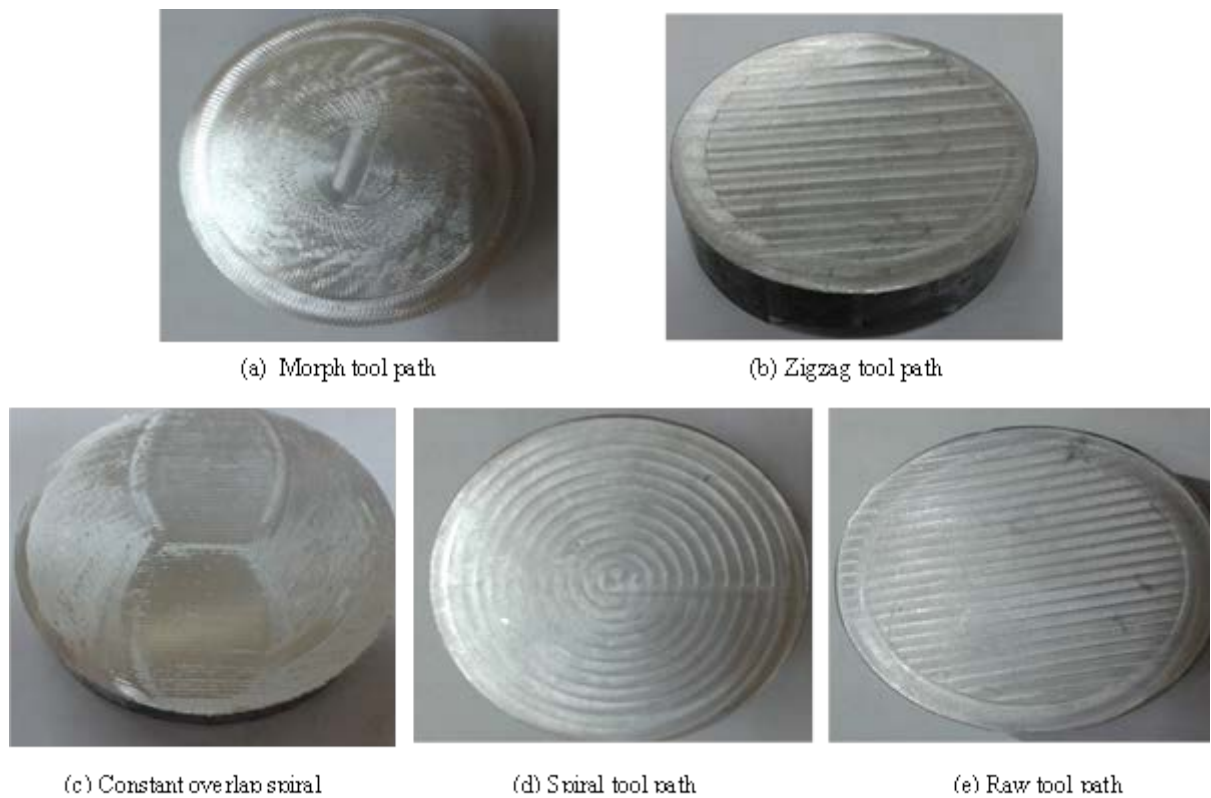
Figure 9: Machined samples using ball end mill tool
