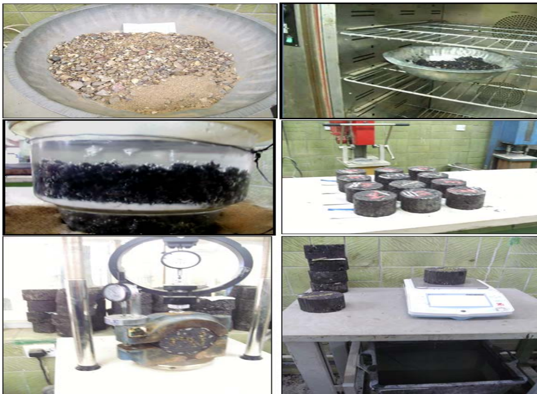
Figure 2: Procedure of testing and sample preparation
