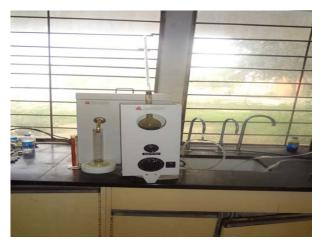
**Figure 1:** Atmospheric distillation unite according to ASTM D -86
