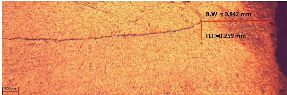
**Figure (17)** microstructures of a friction stir spot weld made using cylindrical pin 800-rpm tool rotational speed.
