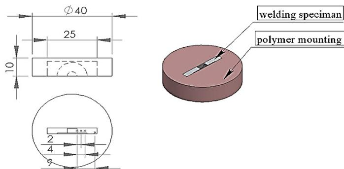
**Figure 8:** Positions of the micro hardness test. (All dimension in mm).
