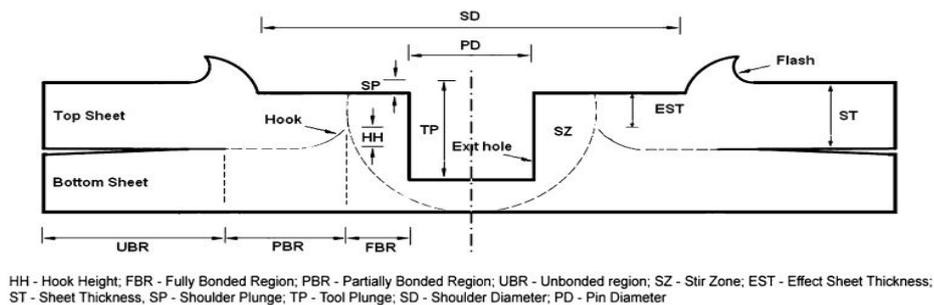
**Figure 2:** Schematic cross-sectional view of a friction stir spot weld [2].
