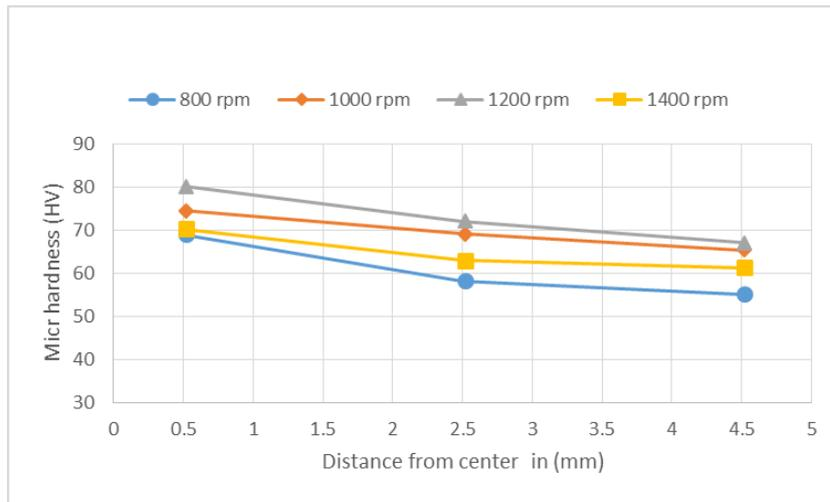
Figure 10: Microhardness profile of welds with triangular pin at different rotational speeds
