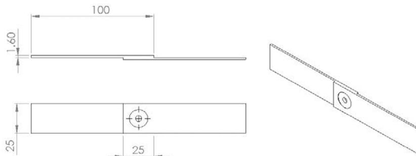
**Figure 3:** Dimensions of the tensile test specimen. (All dimension in mm).
