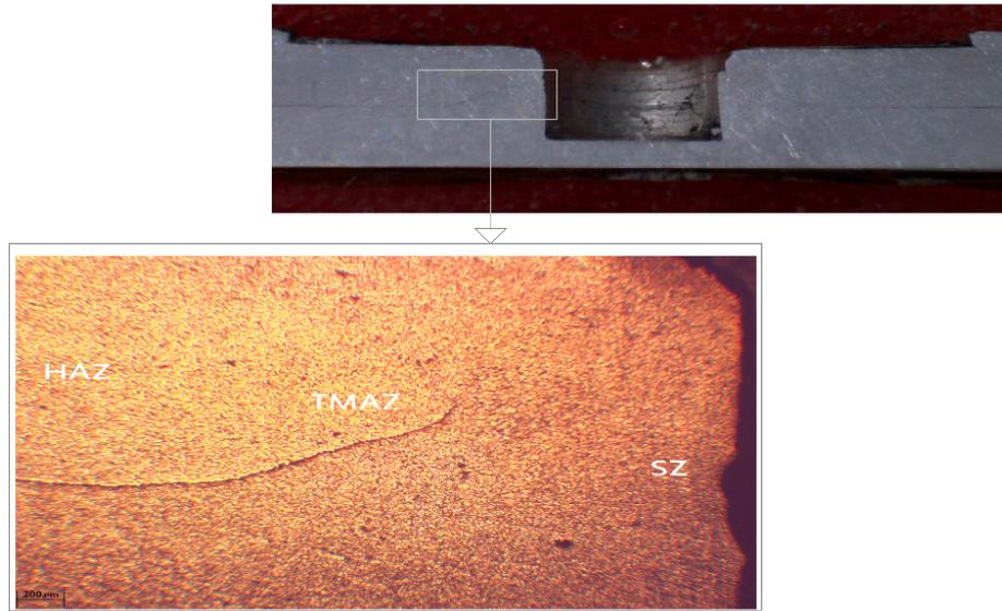
**Figure 14:** Macro- and microstructures of a friction stir spot weld made using triangular pin 1000-rpm tool rotational speed.
