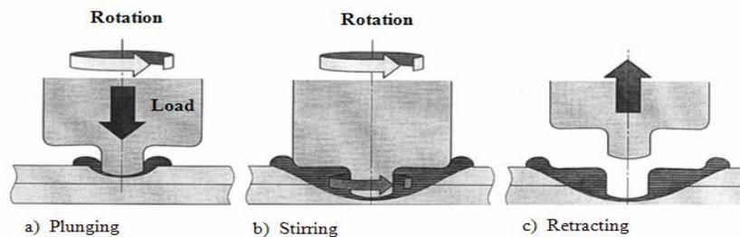
**Figure (1)** Friction stir spot welding (FSSW) process [1]
