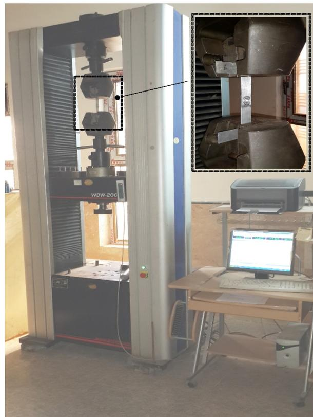
**Figure 6:** Computerized universal tensile testing machine (United Hydraulic SHFM Series).
