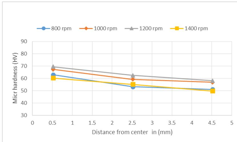
Figure 12: Microhardness profile of welds with tapered pin at different rotational speed,
