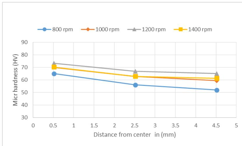
Figure 11: Microhardness profile of welds with cylindrical pin at different rotational speeds
