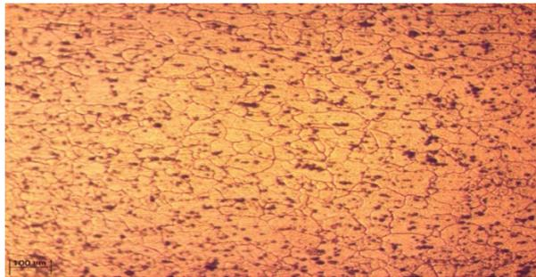
**Figure 13:** Microstructures of AA6061-T6 base material.
