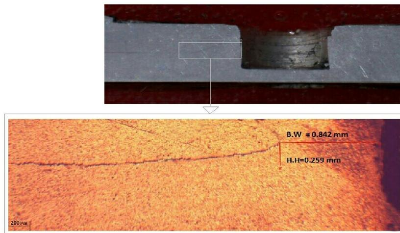
**Figure 15:** Macro- and microstructures of a friction stir spot weld made using triangular pin 800-rpm tool rotational speed.
