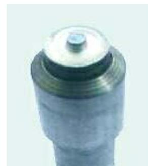
**Figure 6:** Tapered pin tool (All dimension in mm)
