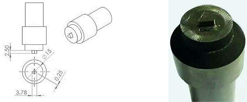
**Figure 7:** Triangle pin tool (All dimension in mm)
