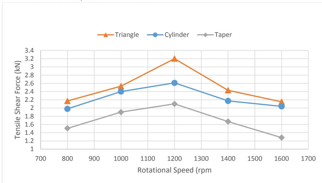
Figure 9: Tensile shear loads at different pin profile and rotational speed
