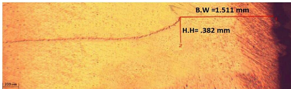
**Figure 16:** microstructures of a friction stir spot weld made using triangular pin 1200-rpm tool rotational speed.
