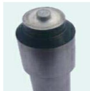
**Figure 5:** Cylindrical pin tool (All dimension in mm).
