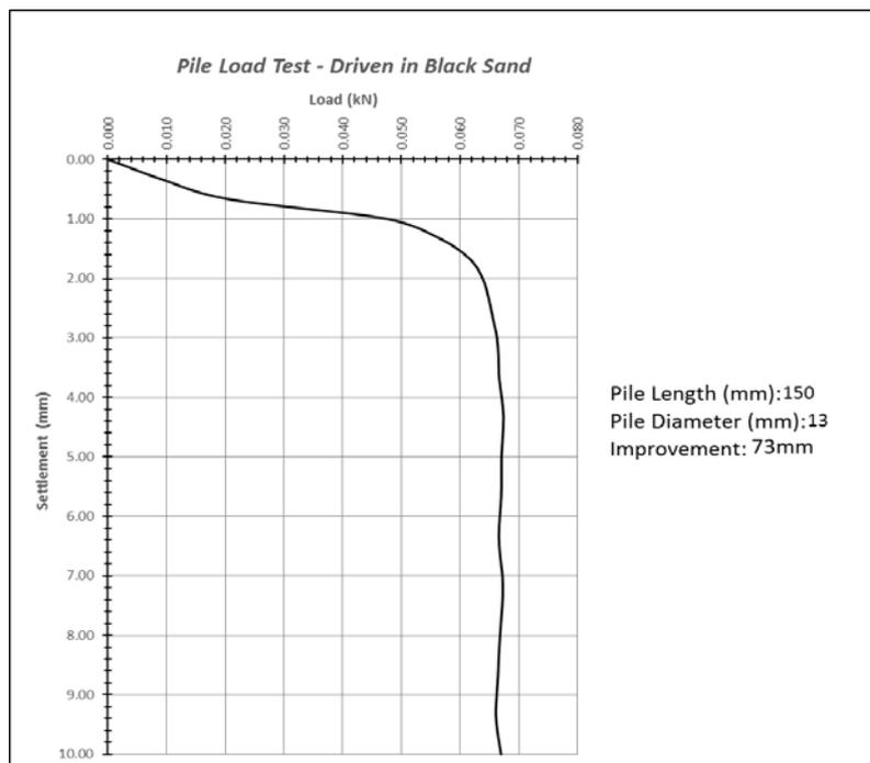
**Figure 5:** pile model length (150mm) diameter of improvement(73mm) estimated pile load capacity(0.067 kN)
