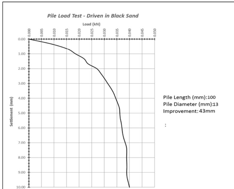
**Figure 4:** Pile model length (100mm) diameter of improvement (43mm) estimated pile load capacity (0.033 kN)
