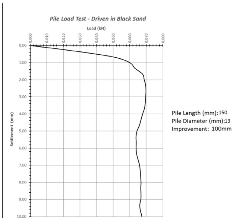
**Figure7:** pile model length (150mm) diameter of improvement(100mm) estimated pile load capacity(0.07 kN)
