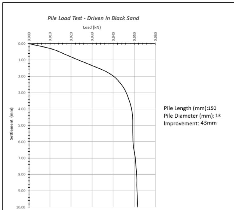
**Figure 3.:** pile model length (150mm) diameter of improvement(43mm) estimated pile load capacity(0.047 kN)
