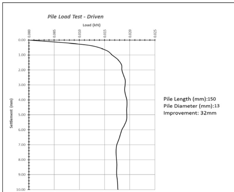
Figure 9: pile model length (150mm) diameter of improvement(32mm) estimated pile load capacity(0.0195 kN)
