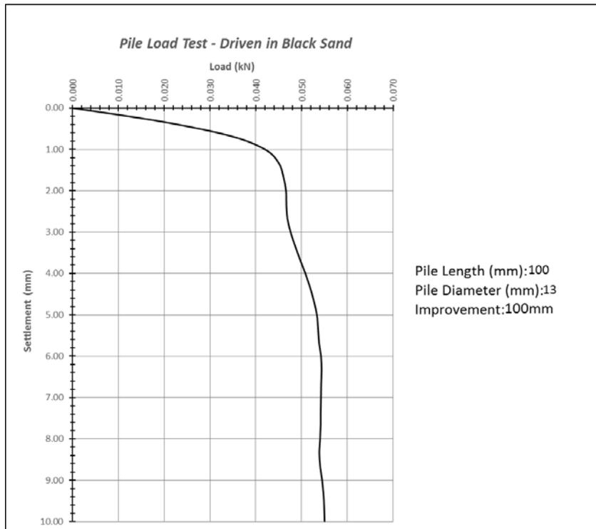
Figure 8: pile model length (100mm) diameter of improvement(100mm) estimated pile load capacity(0.058 kN)
