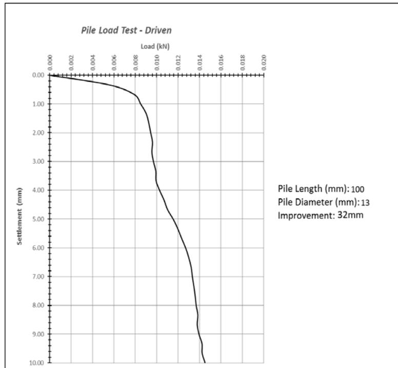
**Figure 10:** pile model length (100mm) diameter of improvement(32mm) estimated pile load capacity(0.0114 kN)
