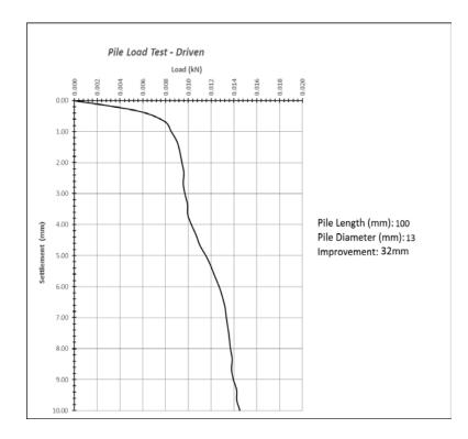
Figure 10: pile model length (100mm) diameter of improvement(32mm) estimated pile load capacity(0.0114 kN)
