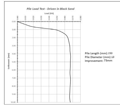
Figure 5: pile model length (150mm) diameter of improvement(73mm) estimated pile load capacity(0.067 kN)
