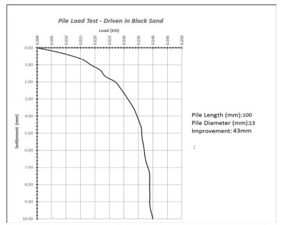
**Figure 4:** Pile model length (100mm) diameter of improvement (43mm) estimated pile load capacity (0.033 kN)
