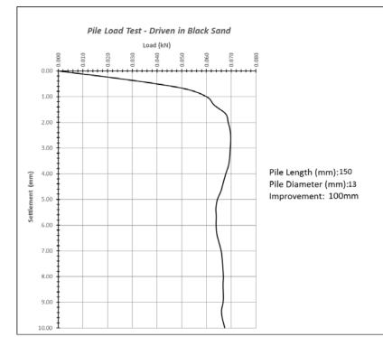
Figure7:. pile model length (150mm) diameter of improvement(100mm) estimated pile load capacity(0.07 kN)
