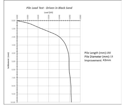
Figure 3:.pile model length (150mm) diameter of improvement(43mm) estimated pile load capacity(0.047 kN)
