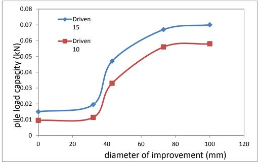
Figure 11: the relation between pile load capacity and diameter of improvement
