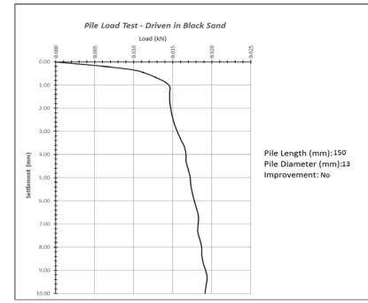
**Figure 1:** pile length 150 mm without improvement estimated pile load capacity(0.015 kN)
