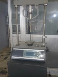
Figure16: Compression device
