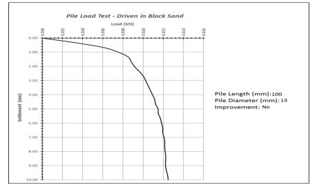
Figure 2:. Pile model length (100 mm) without improvement estimated pile load capacity(0.0095 kN)
