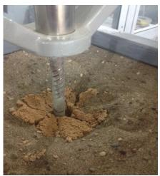
**Figure 15:** Collapsing compacting soil block due to driving pile model
