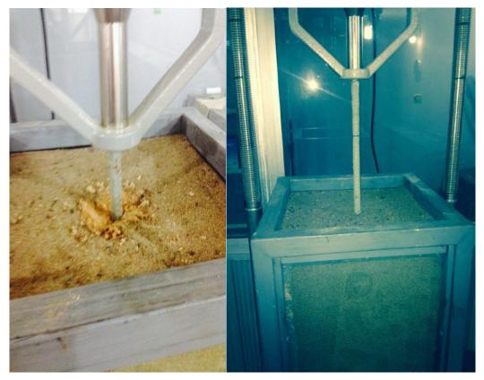
Figure 12: Drive the pile model to require length in both case improvement and without .
