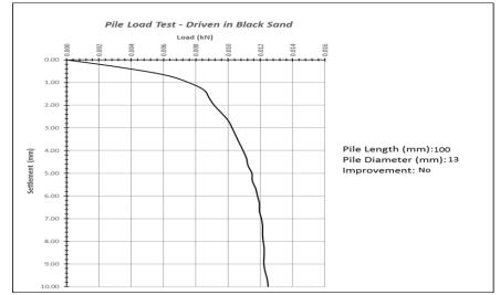
Figure 2:. Pile model length (100 mm) without improvement estimated pile load capacity(0.0095 kN)
