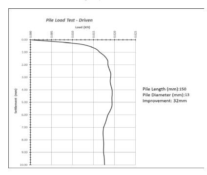
Figure 9: pile model length (150mm) diameter of improvement(32mm) estimated pile load capacity(0.0195 kN)
