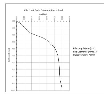
Figure 6: pile model length (100mm) diameter of improvement(73mm) estimated pile load capacity(0.056 kN)
