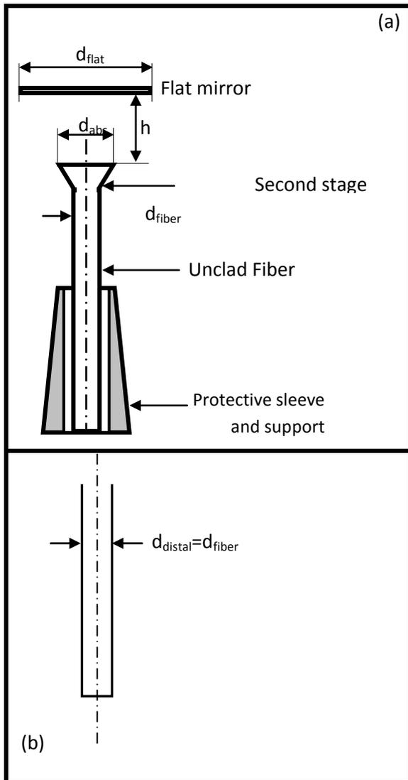
**Fig 4:** In-dish design structure of the second stage (a) Cross section of the fiber absorber where the concentration performed in the dish, (b)Cross section of the distal end of the fiber [5].
