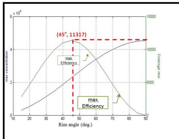
**Figure 3:** The rim half angle effect on the max. concentration and max. efficiency of the parabolic dish. It seen that most suitable angle for the max. efficiency is  $45^\circ$ .
