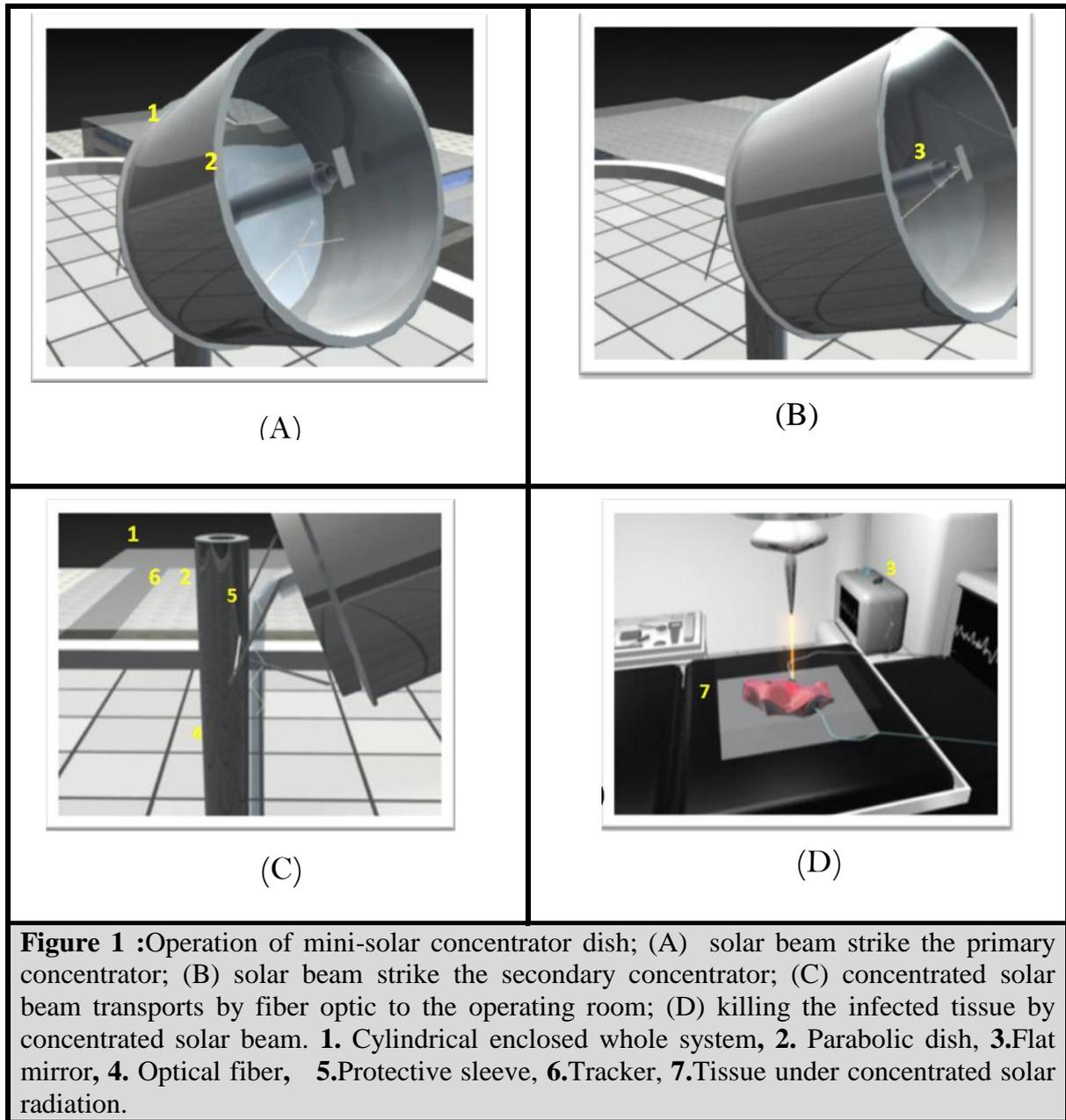
To realize high flux at high efficiency, the design is based on using a parabolic dish primary concentrator with a non-imaging secondary reflector to insure range of solar intensity ( $10^{-1}$  to  $10^{-2}$ )  $Wmm^{-2}$  which is comparable to the necessary laser energy used for surgery especially for cancer cell vaporization.
