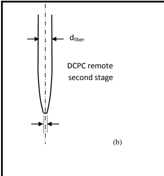
**Fig 5:** Remote design structure of the second stage (a) Cross section of the fiber absorber, (b) Cross section of the distal end of the fiber where the concentration performed remotely in the operating room [5].
