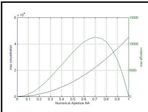
**Figure 7:** Solar concentration as a function of numerical aperture of the fiber of the concentrator system.
