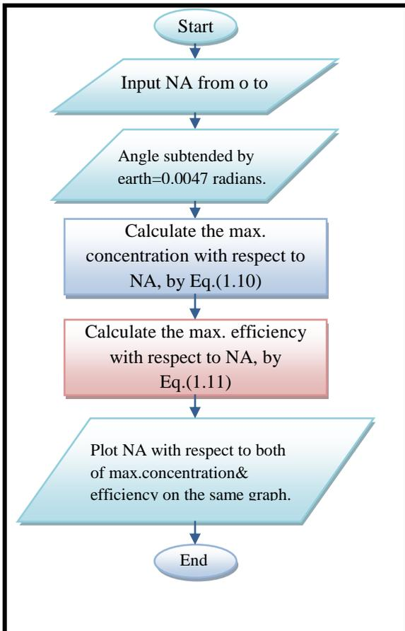
**Figure 6:** Flowchart represents the sequence of MATLAB steps for the concentration as a function of numerical aperture of optical fiber.
