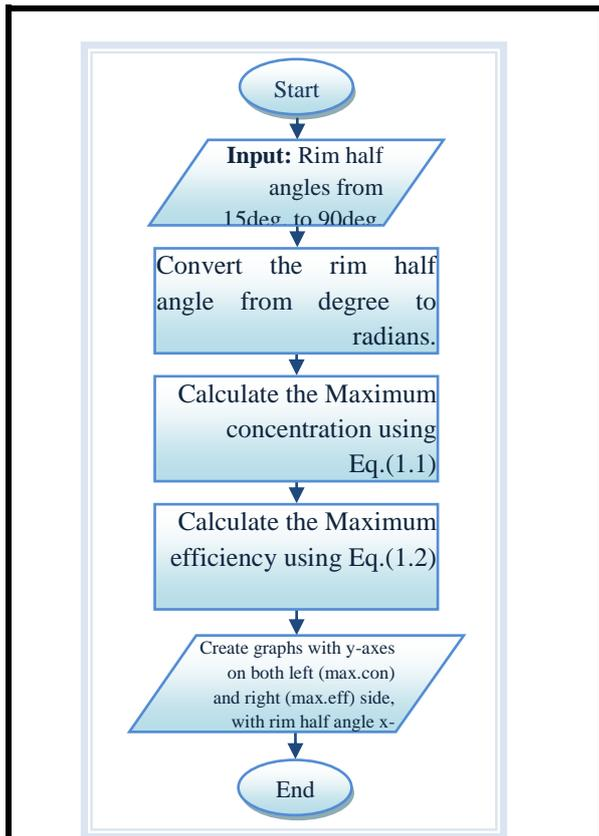
**Figure 2:** Flowchart represents the sequence of MATLAB steps for max. concentration and max. efficiency as a function of rim half angle.
