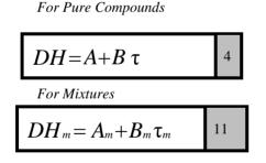
Where DH represents the average reduced saturated enthalpies at any temperatures divided by the average reduced saturated enthalpies at the normal boiling point. The terms DH and  $\tau$  are defined as follows:
