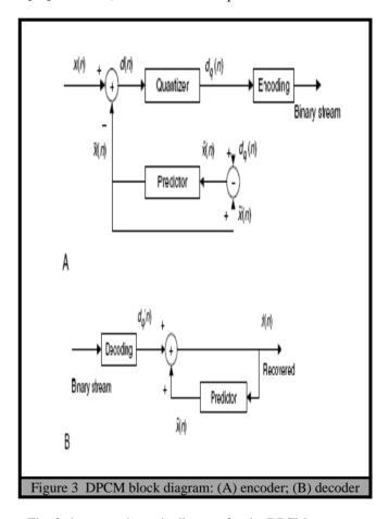
Fig. 3 shows a schematic diagram for the DPCM encoder and decoder. We denote the original signal x(n); the predicted signal x(n); the quantized, or recovered signal  $^x(n)$ ; the difference signal to be quantized d(n); and the quantized difference signal dq(n). The predictor uses the past predicted signal and quantized difference signal to predict the current input value x(n) as close as possible. On the other hand, the decoder recovers the quantized
