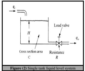
For the liquid level system in Fig.(2). It can be obtained a Mathematical Model to get the relationship between  $q_i$  and  $q_o$  or between  $q_i$  and  $H_{.}[8]$ .
