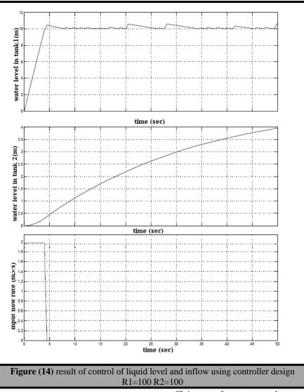
From fig (14) one can notice that, the level in tank1 doesn't increase of ten meters and the input will be close from 2 to zero when the water level will reach to 10m at 4 sec. A series of tests using in the system by changing the parameters R1, R2 and show the comparative result and
