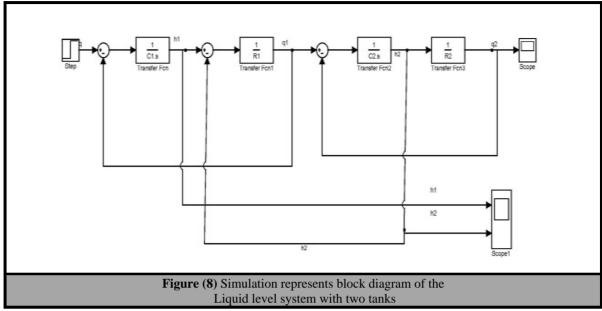
In the simulink, simulate inflow rate to tank 1  $(Q=2 \text{ m}^3/\text{s})$  as a step input is 2 and step time is zero. Let cross section area in tank 1 (C1) equals 0.785 m<sup>2</sup> and in tank 2 (C2) is equal 0.635 m<sup>2</sup> (C1 and C2 is constant) in this design. Firstly assume the Resistivity parameters equal (R1=100 s/m<sup>2</sup>, R2= 100 s/m<sup>2</sup>). It must be
