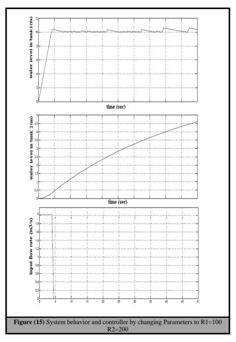
From fig (15), When a scope1 trajectory is finished the change in the resistivity parameter (increasing R2) from 100 to 200 in the system will cause increasing of height in tank2 (R2)
