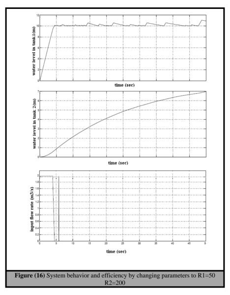
From fig.(16) (case3), The changing in the parameters will cause change in the level in tank2 which reach to 7 m and input will close and open more than time.
