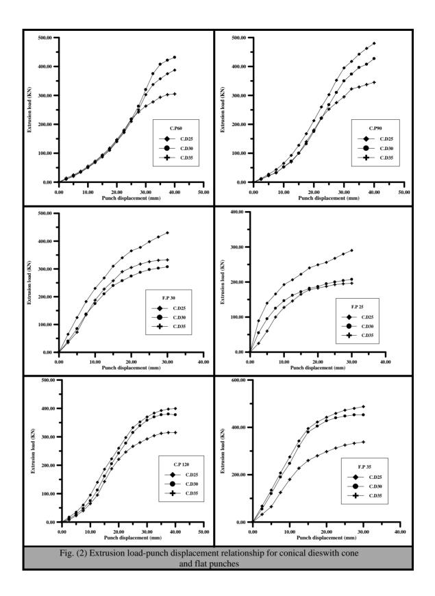
In the flat dies of the reduction area (0.395, 0.555, 0.691), also the load is lowered after it reaches a maximum value before the stroke end except the F.D25 where , the load is continuing to rise to the end of stroke with the punches C.P90,F.P30 and F.P35 as shown in Fig. (3). The reason for continual rising load is to the metal flow restriction forward and dead
