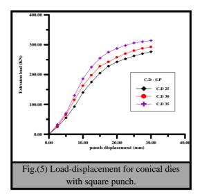
In the square punch which has the same reduction area the extrusion load is increased when the reduction area of die decreases from the beginning of the stroke. This is due to the friction condition which increases when the number of polygonal sides decreases [9], as the friction strongly affects the force in the backward extrusion [14], so the effect of friction at forward die decreases and the shear component of extrusion power increases when the reduction area of conical die decreases.
