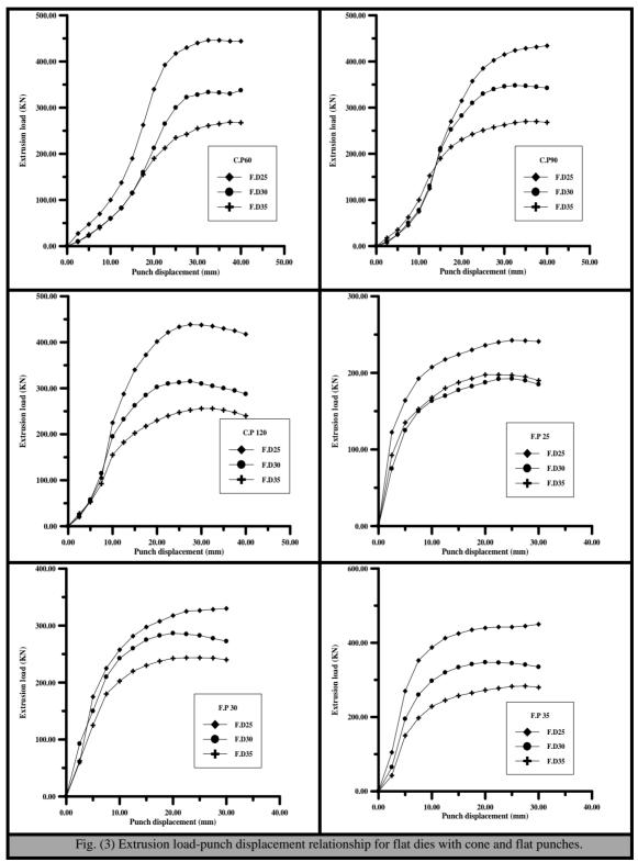
For the conical converged and flat dies, the lower extrusion load appears with reduction area (0.395) of those dies which means that when the reduction area of die decreases the maximum extrusion load decreases too in those dies in the same stroke.
