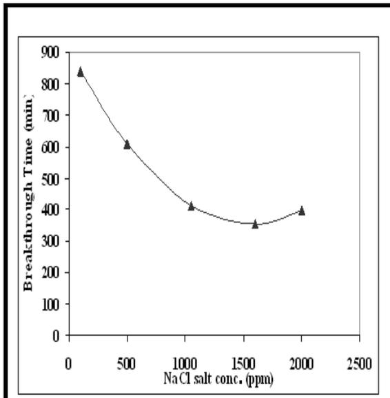
Fig. (3) Effect of NaCl concentration on breakthrough time
