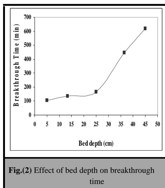
Fig.(2) Effect of bed depth on breakthrough time
