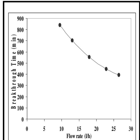
Fig. (4) Effect of Flow Rate on breakthrough time
