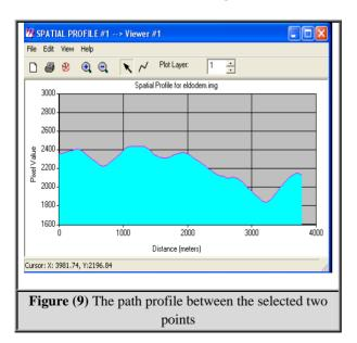
Determine the surface profile for the region containing the selected two points to get an idea about the topology surrounding these two points as shown in Figure (10).
