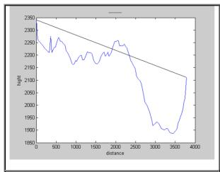
**Figure (14)** Line-of-sight and path profile between points A and B1.
