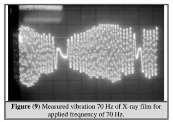
These results show that the two panels behave as linear systems when the ratio between the applied frequency of acoustic wave and the natural frequency is greater than two (or less than one half), so that, the panels may vibrate with same frequency of applied signal. On the other hand, the two panels behave as nonlinear system when the ratio between
