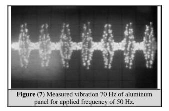
As well, Table 3 shows that X-ray film behave as a linear system when the applied frequency departs from natural frequency region, while the system becomes nonlinear when the applied vibration approaches the natural frequency.
