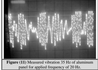
the applied frequency of acoustic wave and the natural frequency is less than two (or greater than one half). This conclusion is in good agreement with the phenomenon of partially damped resonance vibration presented by Thomson [4], and is depicted in figure 12 with arbitrary scale.
