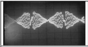
Figure (6) Measured vibration 22.8 Hz of aluminum panel for applied frequency of 20Hz
