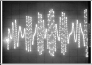
Figure (10) Measured vibration 49 Hz of aluminum panel for applied frequency of 40 Hz.
