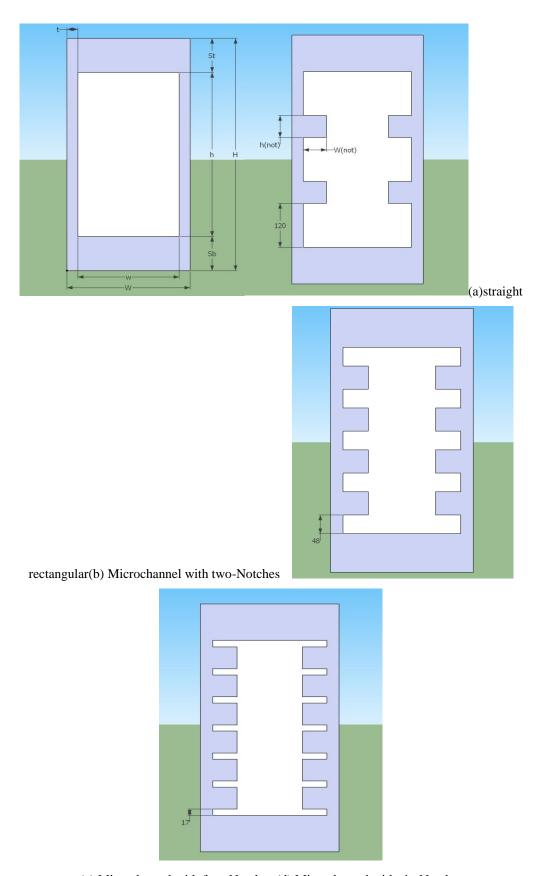
(c) Microchannel with four-Notches (d) Microchannel with six-Notches **Figure 2:** straight and with notches microchannels
