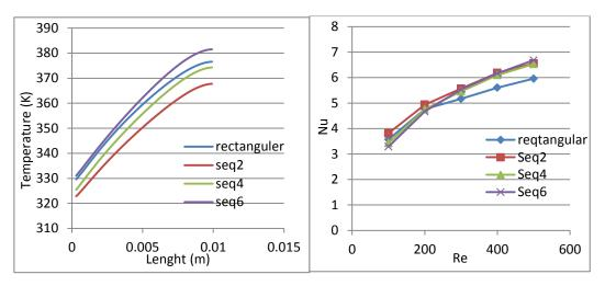
**Figure 9:** Variation on fluid temperature for pure water, at (Re=100) & (Q =150) W/cm<sup>2</sup> at bottom channel wall
