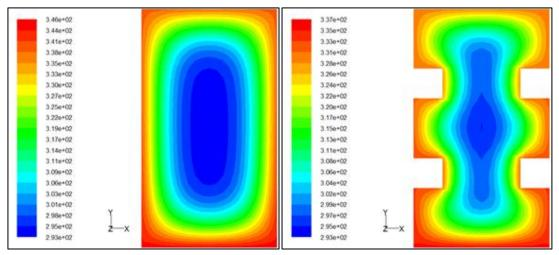
**Figure 5:** Temperature contour of Outlet at q=150W/cm<sup>2</sup> and Re=300
