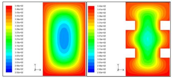
**Figure 3:** Temperature contour of Outlet at q=100W/cm<sup>2</sup> and Re=100
