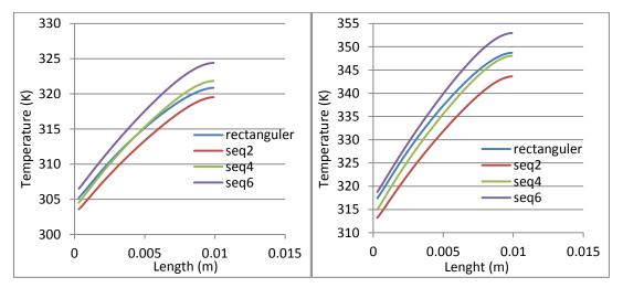
**Figure 7:** Variation on fluid temperature for pure water, at (Re=100) & (Q=50)W/cm<sup>2</sup> at bottom channel wall
