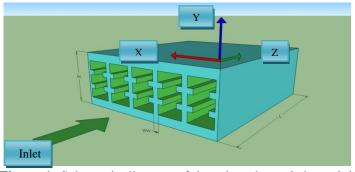
Figure 1: Schematic diagram of the microchannels heat sink
