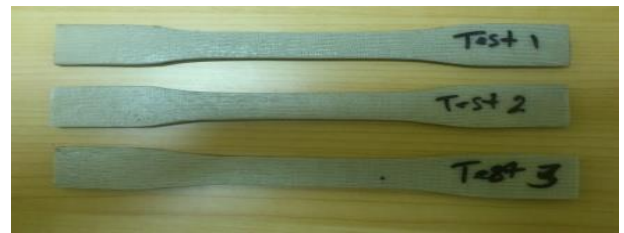
Figure 4: The general shape of tensile specimen of designed material.
