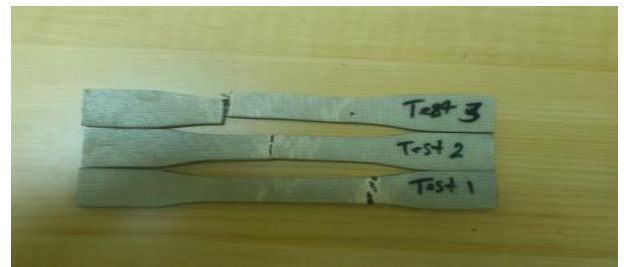
Figure 5: Tensile test specimens of designed material after test.
