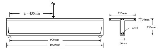
Figure 3: Dimensions and Details of Tested T-Beams
