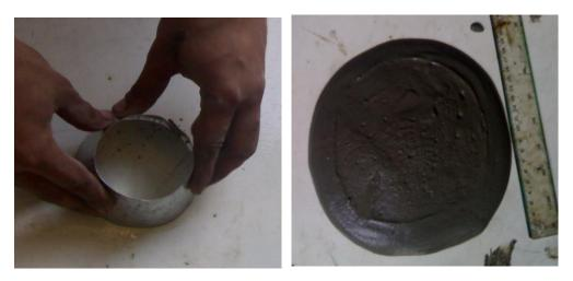
Figure 1: Consistency test by Flow Table
