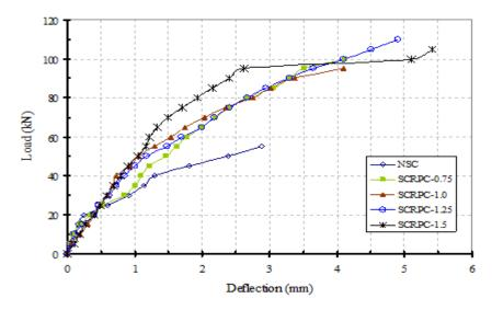
Figure 6: Load-Deflection Relationship for Tested beam Specimens
