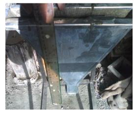
Figure 2: Viscosity and fillingability by V-funnel flow time test
