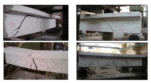
Figure 5:Crack Patterns for T-Beams
