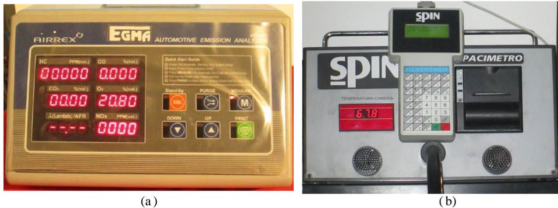
Figure 3: Emission detecting devices (a) Gas analyser (b) Smoke meter
