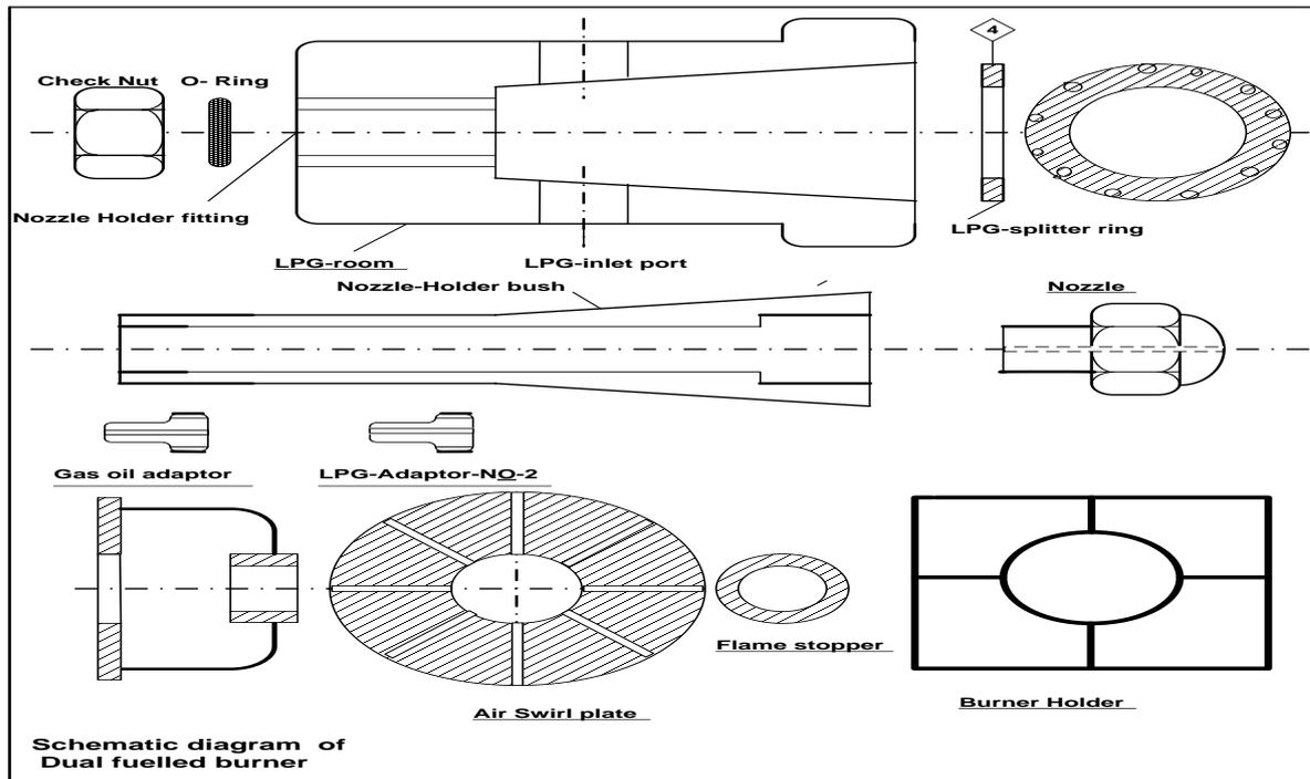
Figure 2: Schematic diagram of the dual fuel burner.
