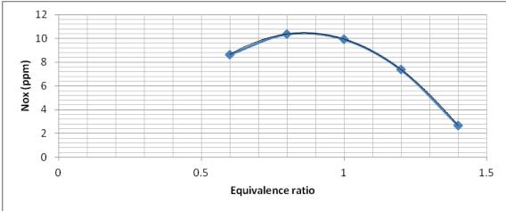
Figure 8: Thermal load (29.7 kW)
