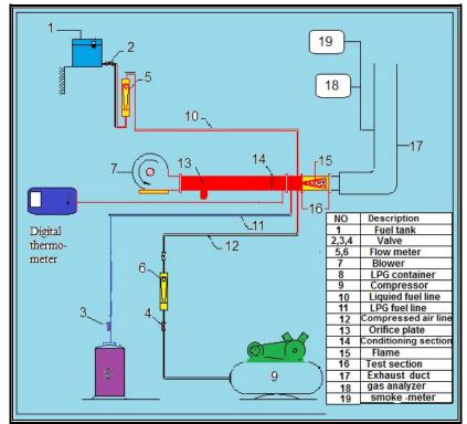
Figure 1: The test rig.
